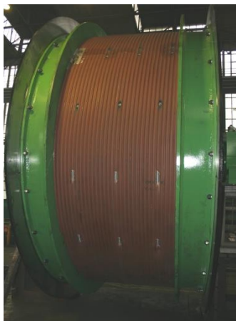
Fig. 5. Winding drum with a steel, grooved lining installed on the drum shell
