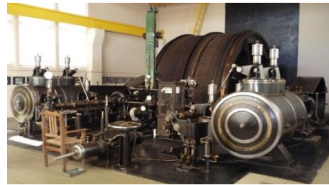
Fig. 4. Steam double-drum hoisting machine Museum of Bochnia Salt Mine [2]
