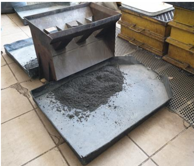
Fig. 1. Averaging the furnace slags by the sample divider
