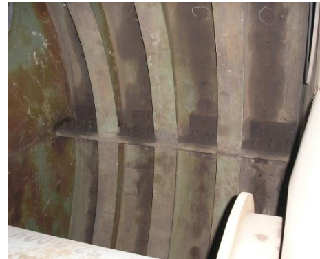
b) shell with circumferential ribs
