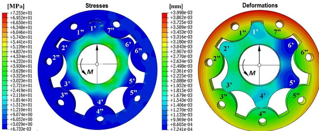
Fig. 6. Distribution of reduced stresses and deformations in a cycloidal wheel assembly according to the new solution
