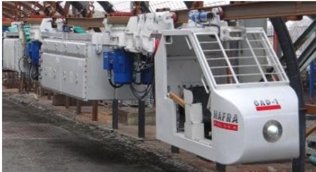
**Fig. 6.** Haulage unit of the GAD-1 suspended monorail [9]
