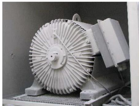
**Fig. 3.** Tests in the dust chamber for conformity with the ATEX Directive – IP code
