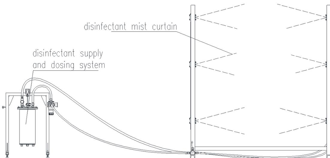
**Fig. 5.** General view of the installation [18]
