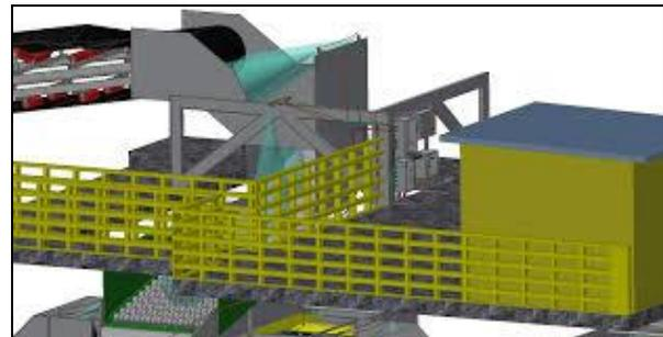
**Fig. 12.** Visualization of a part of the NEPTUN spraying system – a transfer point in the area of raw coal bunkers [13]
