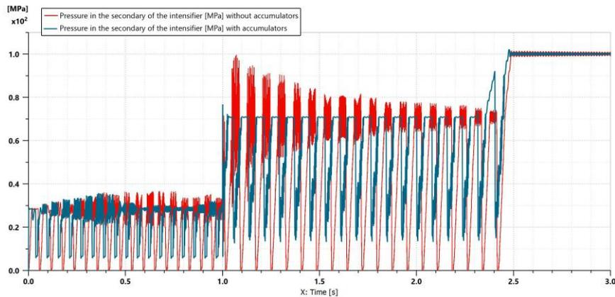
**Fig. 7.** Variation of the pressure in the secondary of the intensifier over time
