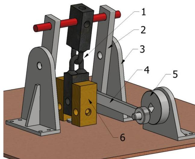
**Fig. 8.** Model of the stand for 3D printing
