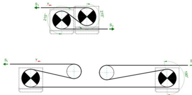
**Fig. 1.** Basic configurations of a two-drum drive [5]
