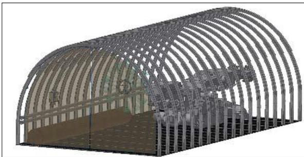
**Fig. 11.** Visualization of the EMZ-BRYZA roadway dust barrier [12]
