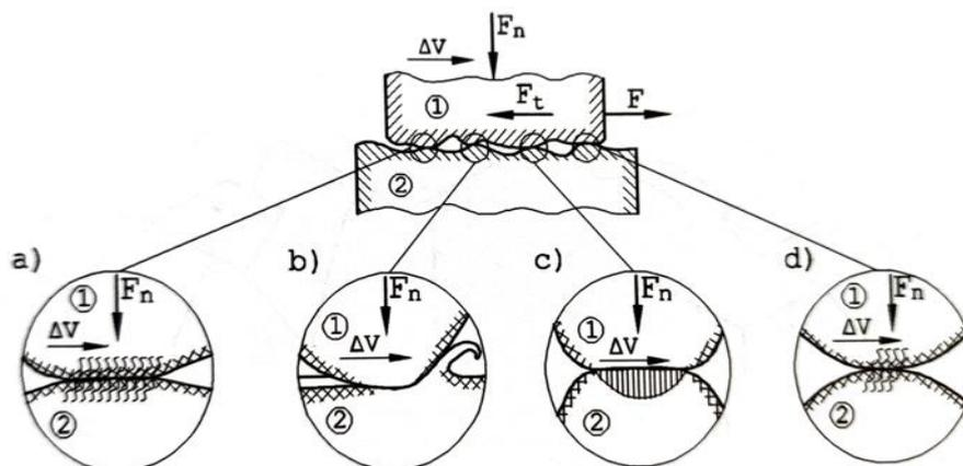
**Fig. 1.** Tribological wear mechanisms (a-adhesive, b-abrasive, c-fatigue, d-corrosion) [1]
