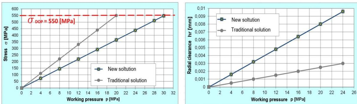
Fig. 7. Change of reduced stresses and deformations depending on the working pressure  $p$  for two types of cycloidal wheels
