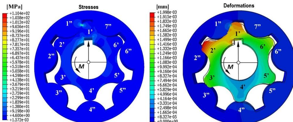
Fig. 2. Distribution of reduced stresses and displacements in a cycloidal wheel assembly
