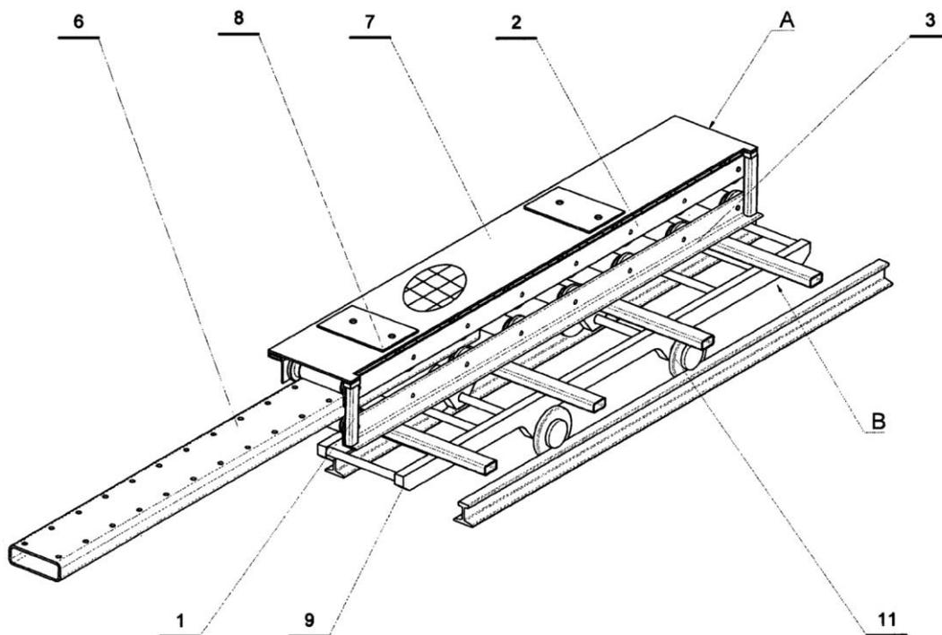
**Fig. 5.** Design of the mobile working platform unit:
