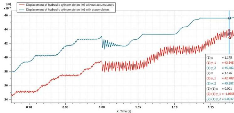
Fig. 12. Detail: displacement of the piston of the hydraulic cylinder
