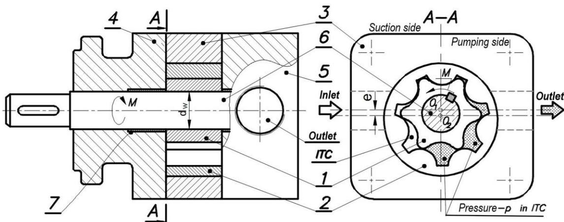
Fig. 1. Design and principle of operation of a hydraulic gerotor machine
