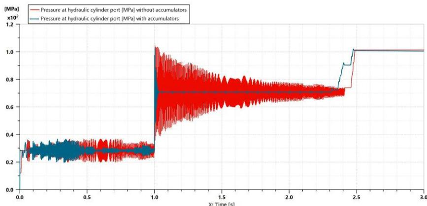
**Fig. 8.** Variation of the pressure at the port of hydraulic cylinder over time
