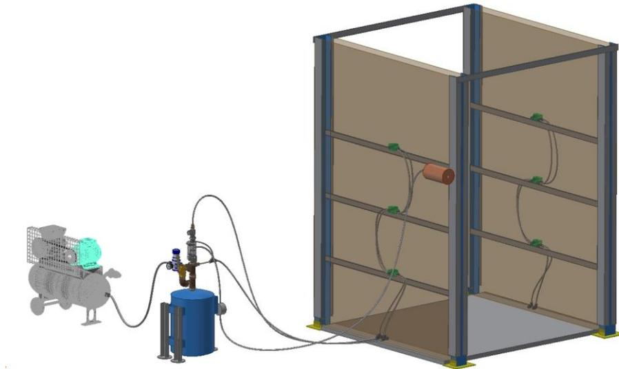
**Fig. 11.** 3D model UMID demonstrative mist disinfecting installation [21]
