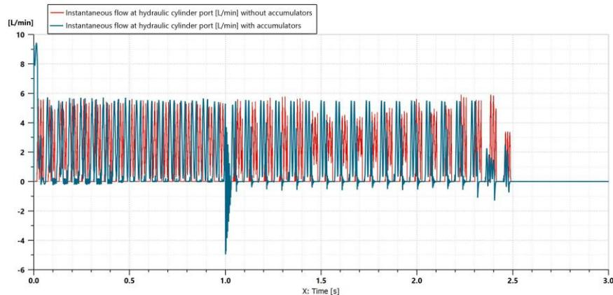
**Fig. 9.** Variation of the instantaneous flow rate at the hydraulic cylinder port over time
