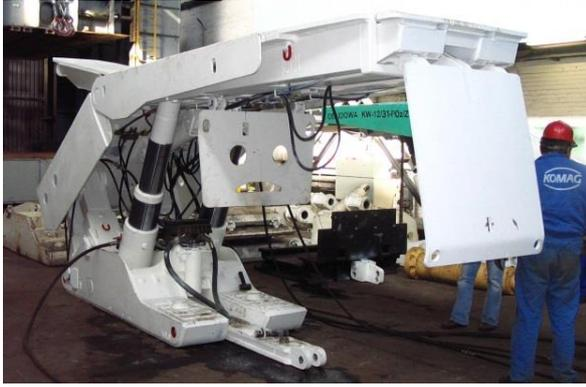
**Fig. 13.** KHW 12/28-POz/Pp powered roof support unit [14]
