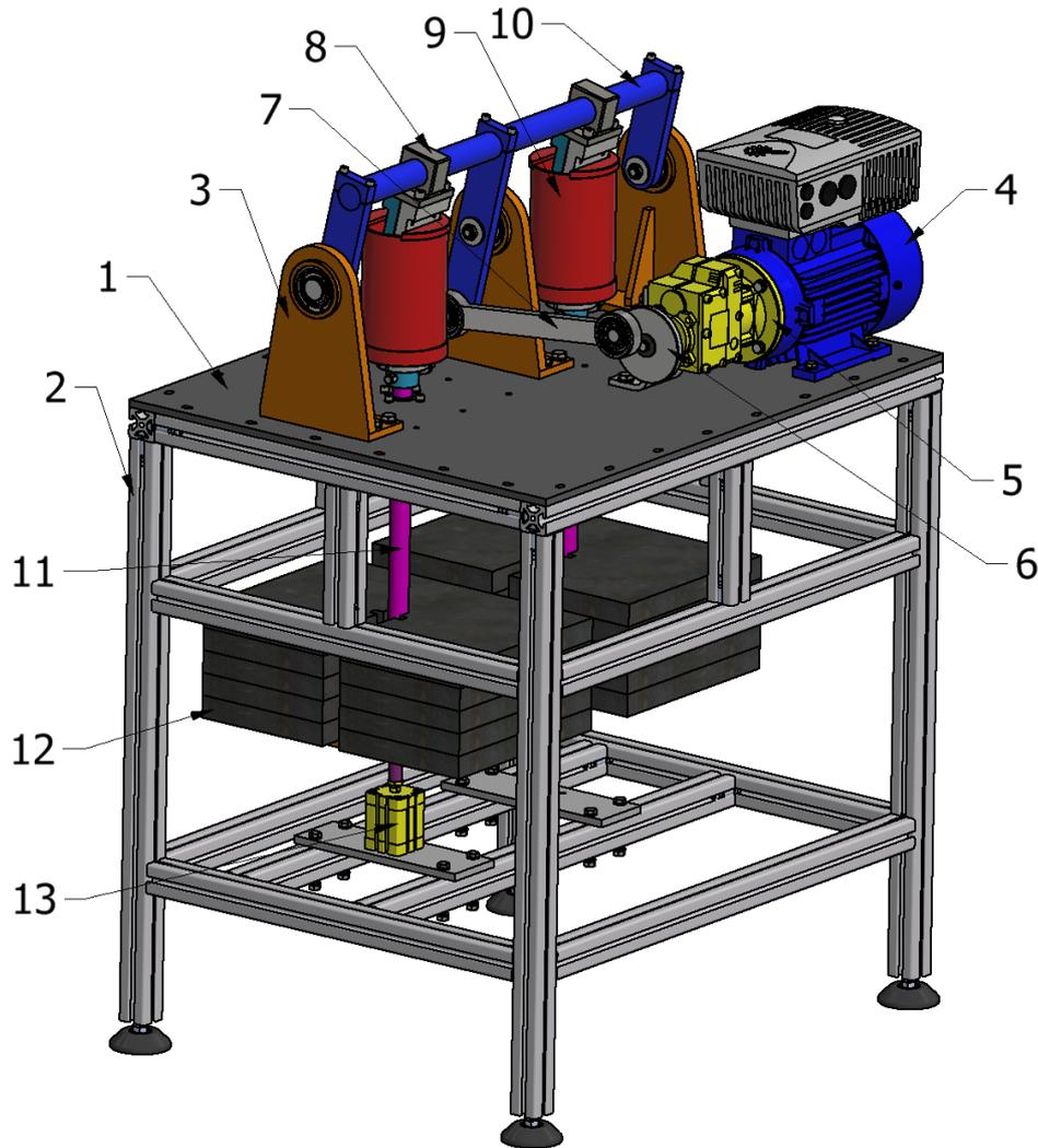
**Fig. 4.** Model of the test stand - general view (1- table top, 2-table frame, 3- stands, 4- electric motor with inverter, 5- reducer, 6-eccentricity (crank), 7-connector, 8-upper link holder, 9 - container for abrasive, 10-rocker arm, 11-load bar, 12-weights, 13-pneumatic cylinder)
