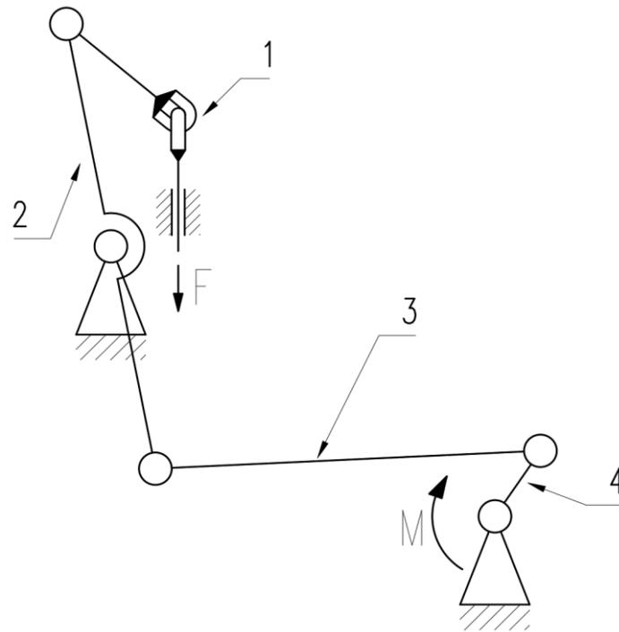
**Fig. 3.** Kinematic diagram of the conceptual test stand
