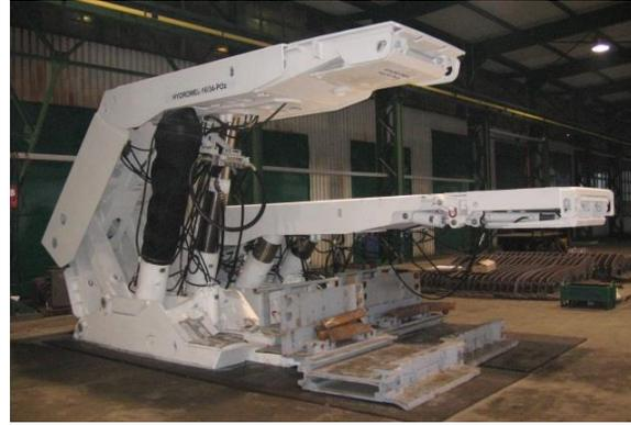
**Fig. 14.** HYDROMEL 16/34-POz powered roof support unit [14]
