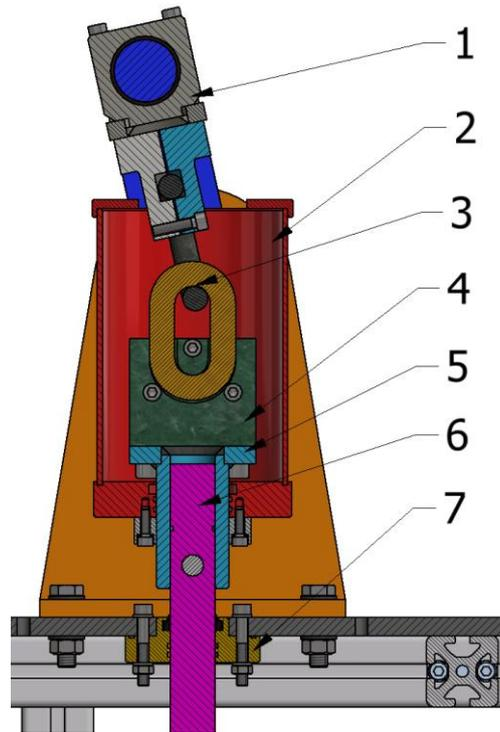
**Fig. 5.** Cross-section of the tank for abrasive
