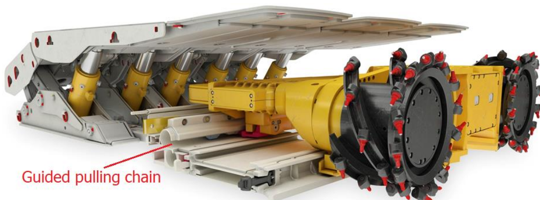
Fig. 11. Polish GUŁ-500 shearer with guided chain haulage system with external drives [20]
