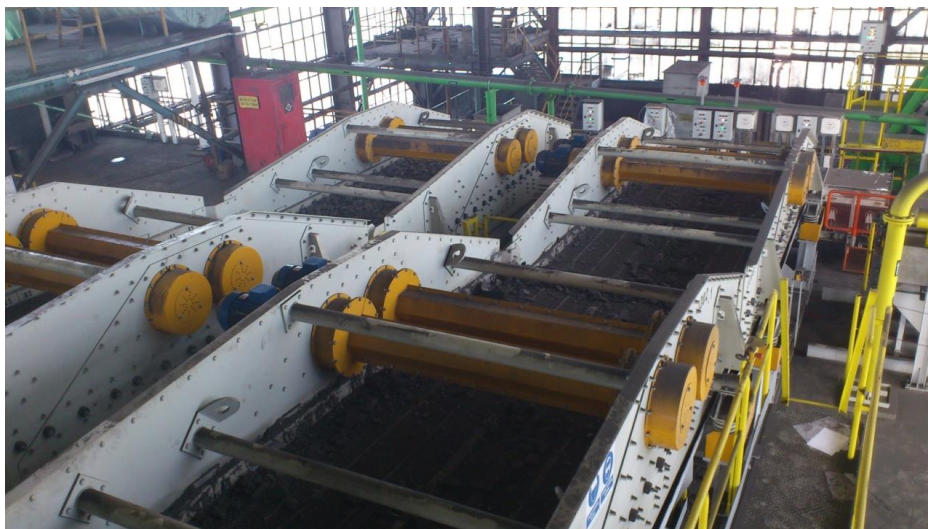
Fig. 5. Two tandem vibrating screens PWP1-2.2x5.25
