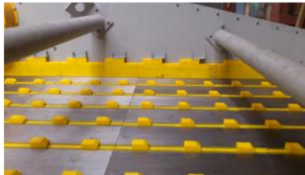
Fig. 14. Sieve deck, slotted, welded, built-in PRO-CLIN system
