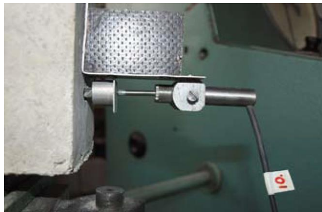
Fig. 3. Fixation of the displacement recorder of the bar end [8]
