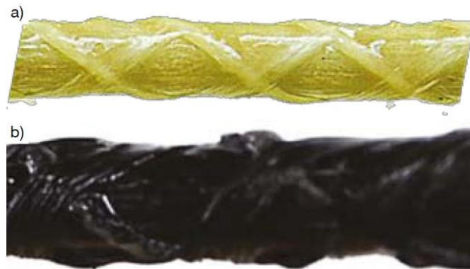
Fig. 9. View of surfaces of composite bars [8] a) GFRP bar, b) BRFP bar
