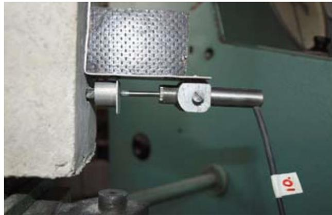
**Fig. 3.** Fixation of the displacement recorder of the bar end [8]
