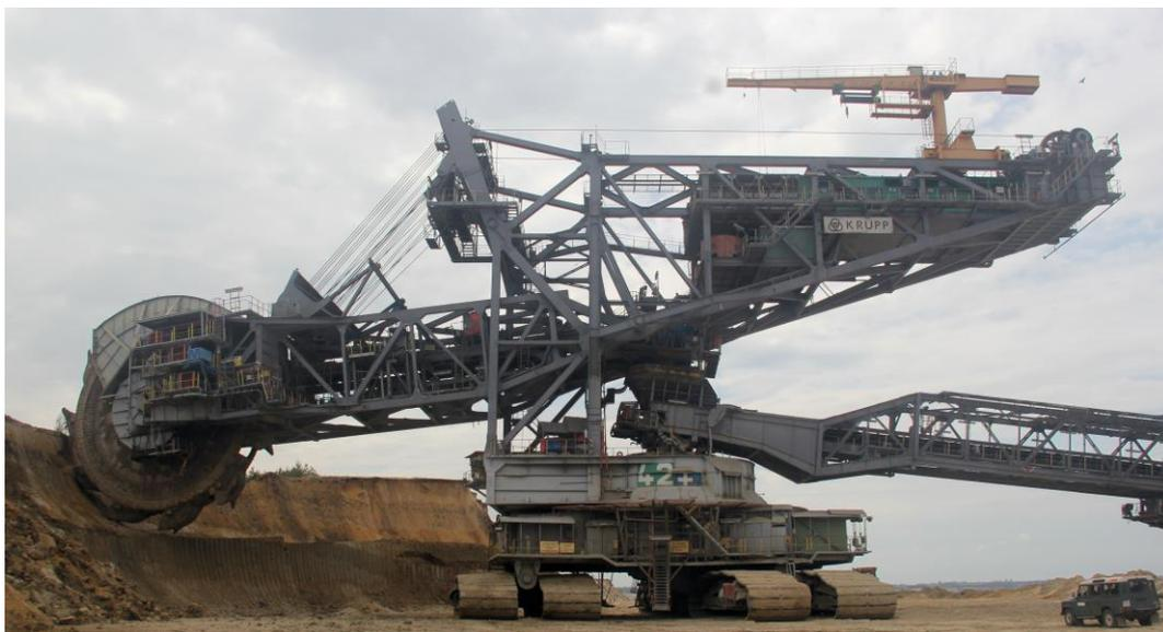
Fig. 1. Bucket-wheel excavator SchRs4600 of KRUPP
