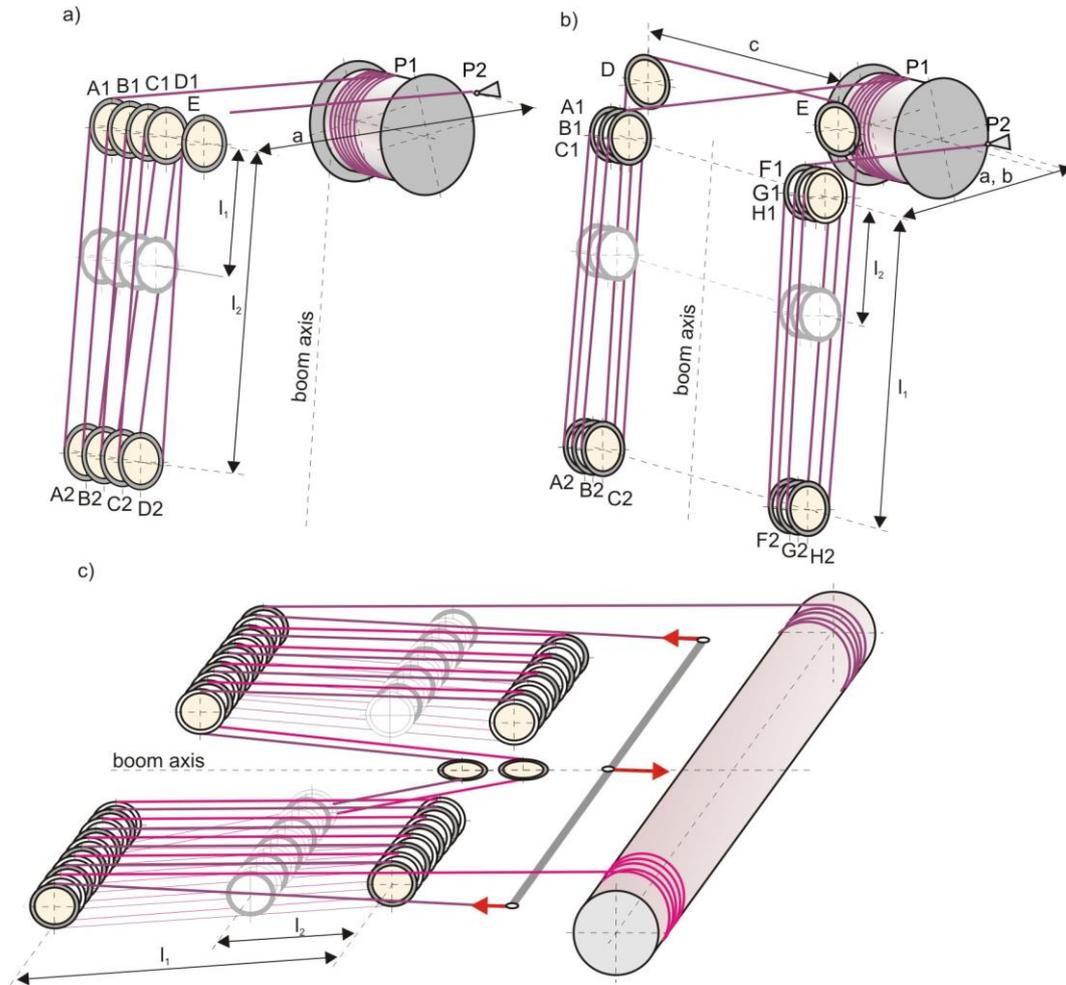
**Fig. 2.** Kinematic diagrams of rigging systems for machines with a cutting wheel:
