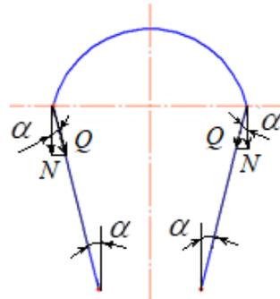
**Fig. 4.** Calculation scheme for determining the resistance in hydraulic props, depending on the angle of their installation: where  $\alpha$  is the angle of installation of hydraulic props;  $Q$  – resistance of hydraulic prop,  $N$
