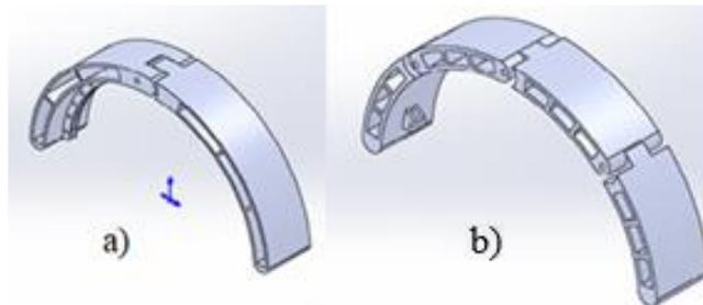
**Fig. 5.** Examples of overlapping devices: a) two-sectional, b) four sectional
