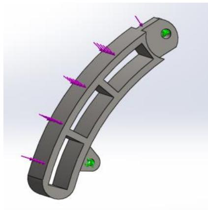
**Fig. 8.** Loading scheme of the 4-sectional overlapping unit
