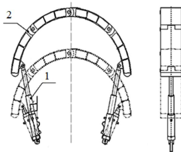
Fig. 1. Hydraulic manipulator of the supporting device:
