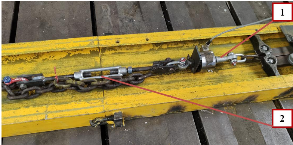
Fig. 5. Measurement sensors, markings: 1- force sensor, 2- turnbuckle
