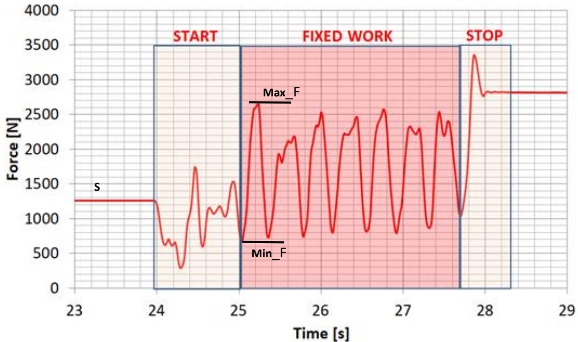
Fig. 16. An exemplary course of dynamic forces for one travel of the measuring head at the basic direction
