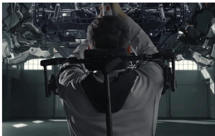
Obr. 11 Hyundai exoskelet – VEX (Hyundai 2023)
