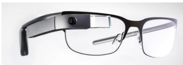
Obr. 17 Okuliare pre Pick by vision technológiu (Ecfeda 2024)
