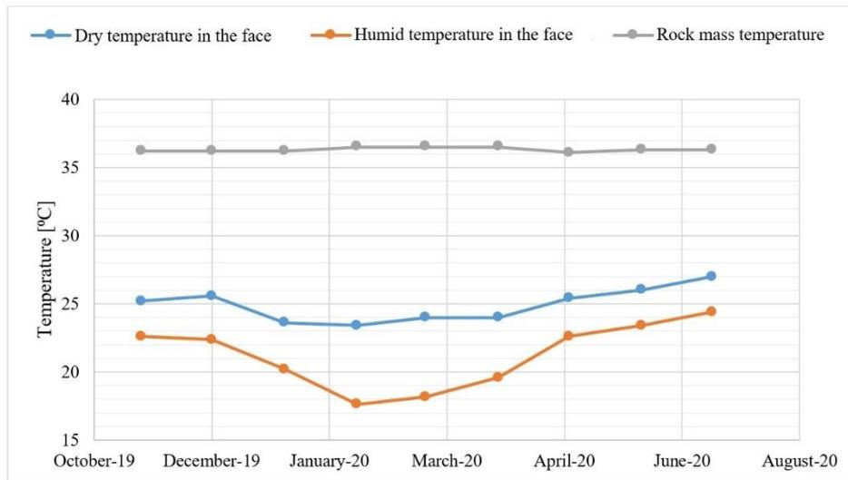
Fig. 11.25. Graph of the temperature changeability in the Bw-1n test roadway [135]
