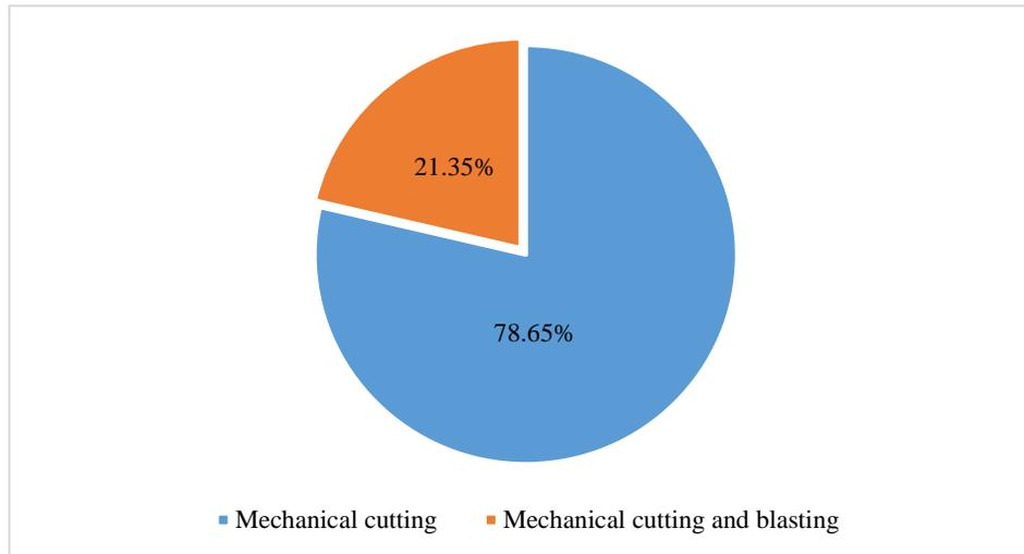
Fig. 6.3. Percentage shares of the workings drivage methods in all the mines of the JSW S.A. in the period 2017-2018
