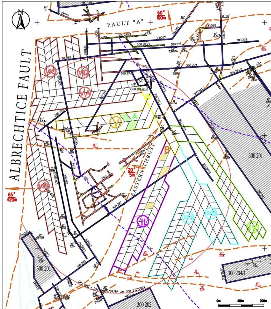
Fig. 3.3. A part of the panel mined with use of the room-and-pillar method [51]
