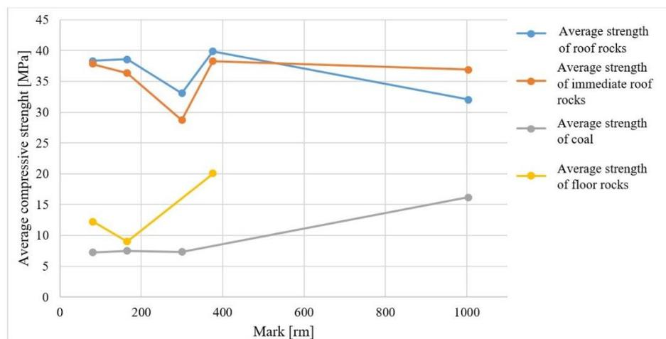
Fig. 8.2. Changeability graph of penetrometric values of the rocks compressive strength at the length of the Bw-1n test roadway [134]
