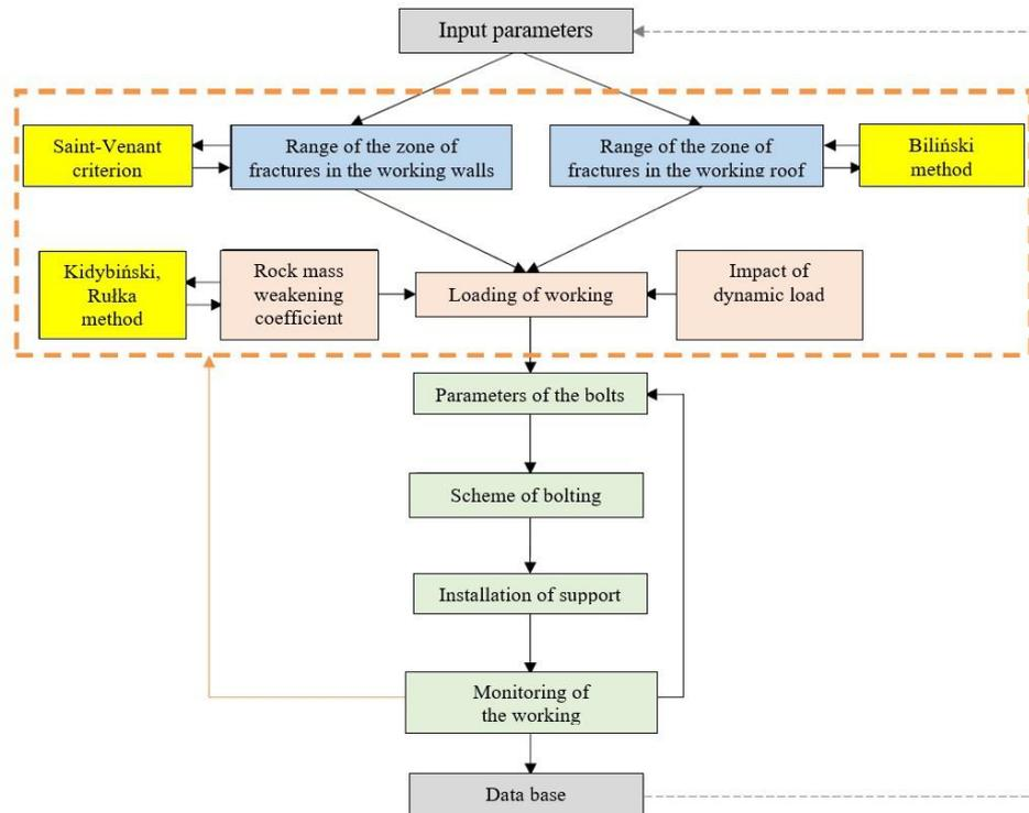
Fig. 10.1. Algorithm of activities during the roof bolting support designing with use of analytical-empirical method [136]
