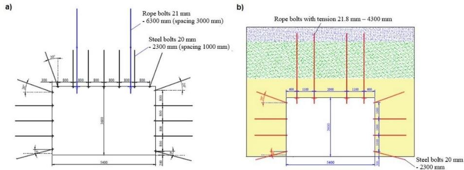
Fig. 3.23. Changes in the bolting system a) originally used b) an application of the BMRET technology [27]
