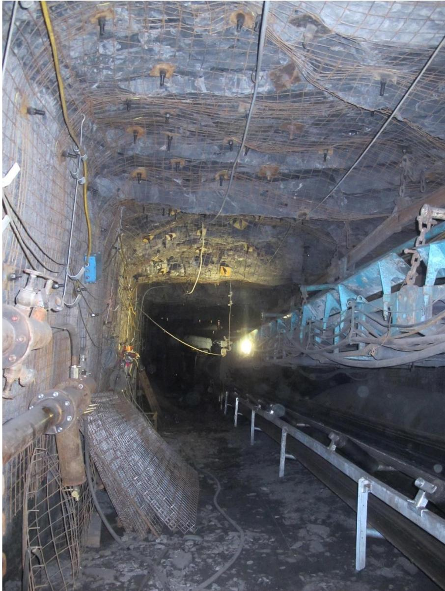
**A view of the suspended belt conveyor cooperating with Bolter Miner 12CM30 in Bw-1n roadway in Budryk coal mine**
