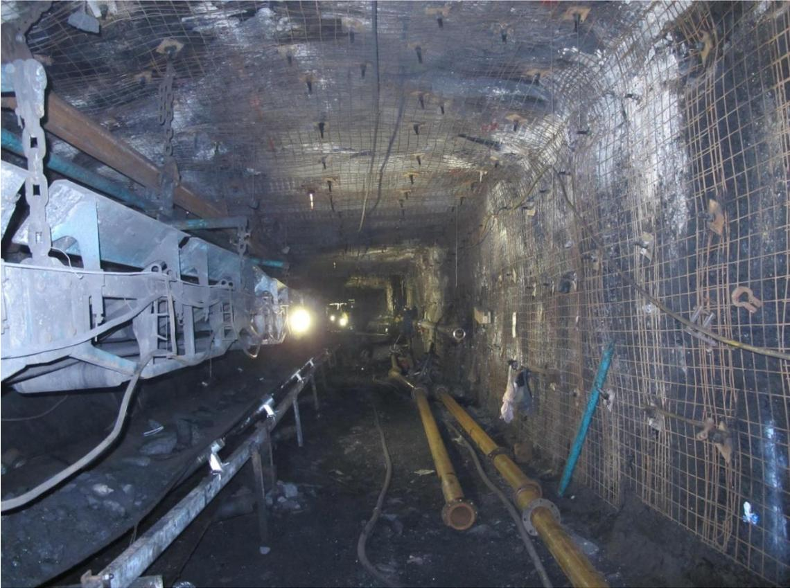
**A view of the suspended belt conveyor cooperating with Bolter Miner 12CM30 in Bw-1n roadway in Budryk coal mine**
