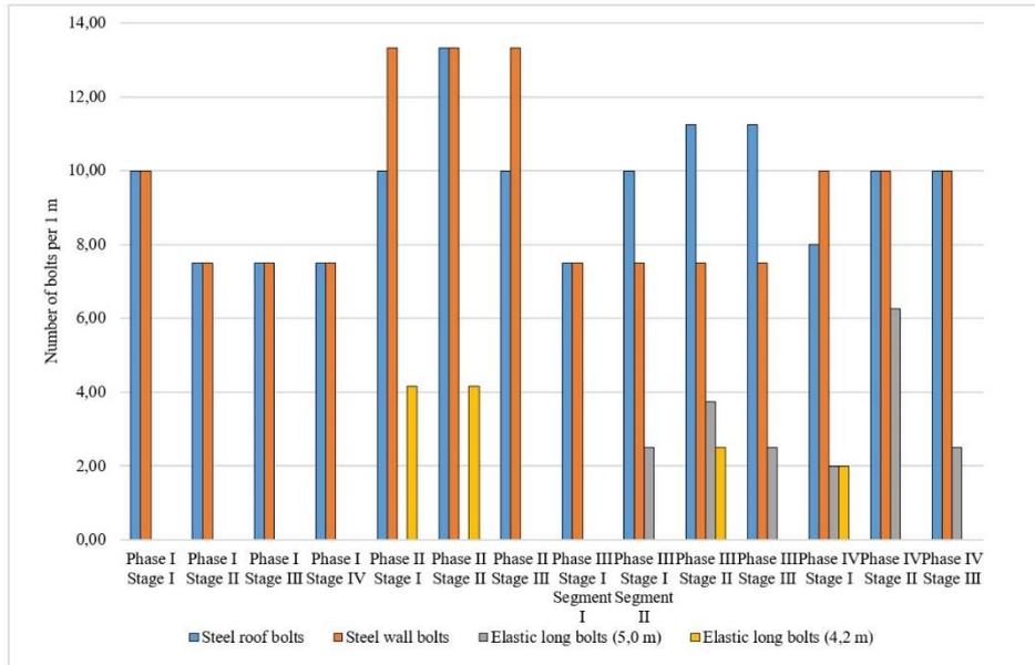
Fig. 11.20. Number of bolts falling to 1 m of the working at individual driving stages of the Bw-1n test roadway
