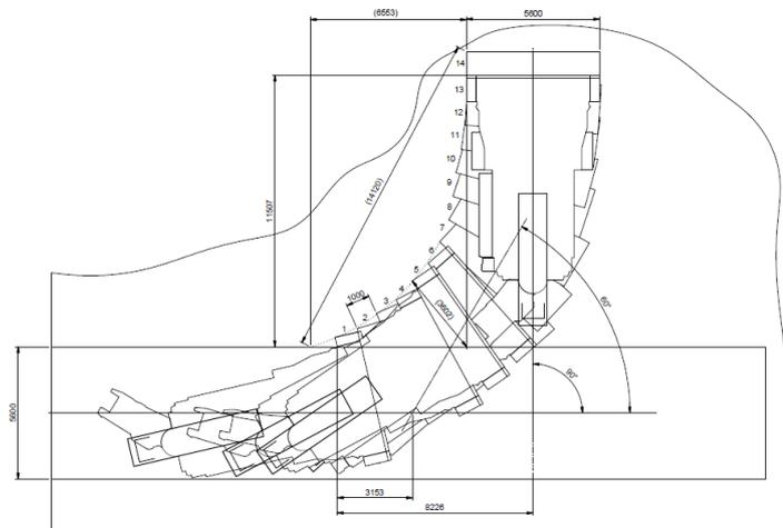
Fig. 13.1. Model of the bend drivage at  $90^\circ$  with use of the 12CM30 machine according to analyses of Komatsu/Joy Global
