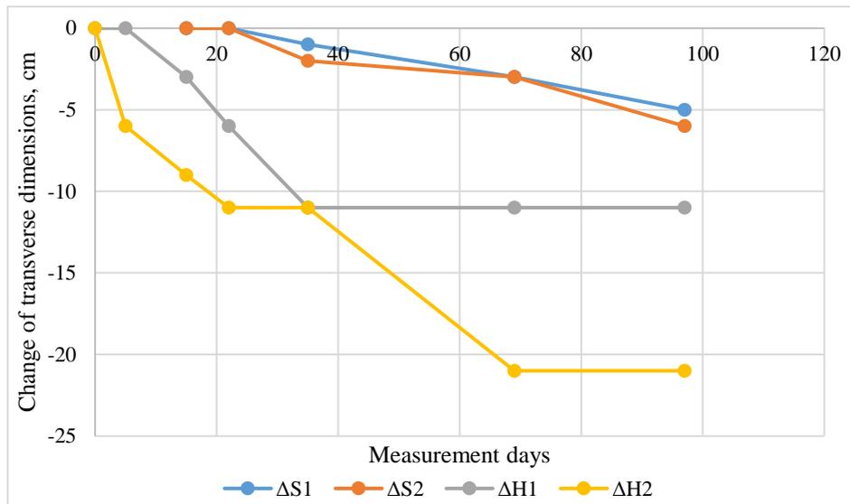
Fig. 12.33. Change of the working transverse dimensions – convergence measuring station No. 5 [135]
