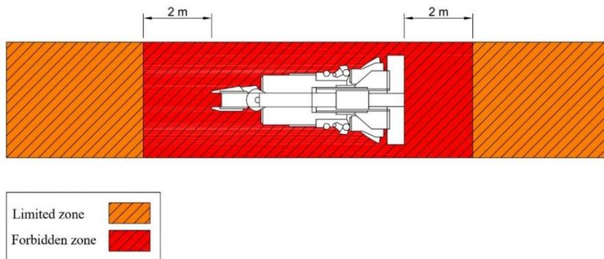
Fig. 11.4. Access zones during the machine advance [130]
