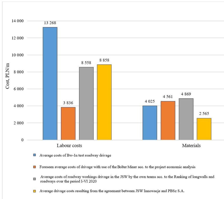
Fig. 14.28. Statement of real and foreseen costs of the Bw-1n test roadway drivage [128]
