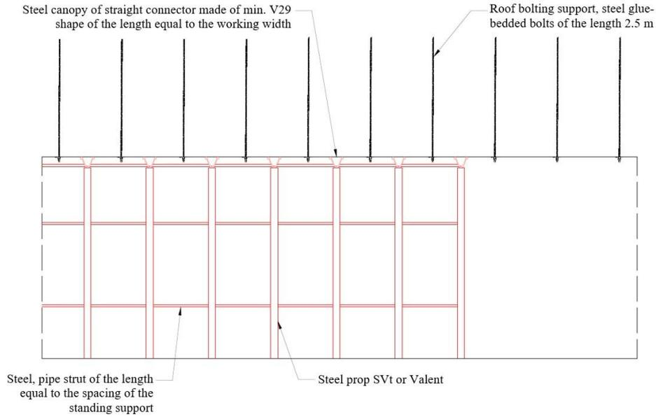
Fig. 11.10. Scheme of the working protection at Stages I-III of Phase I [138]
