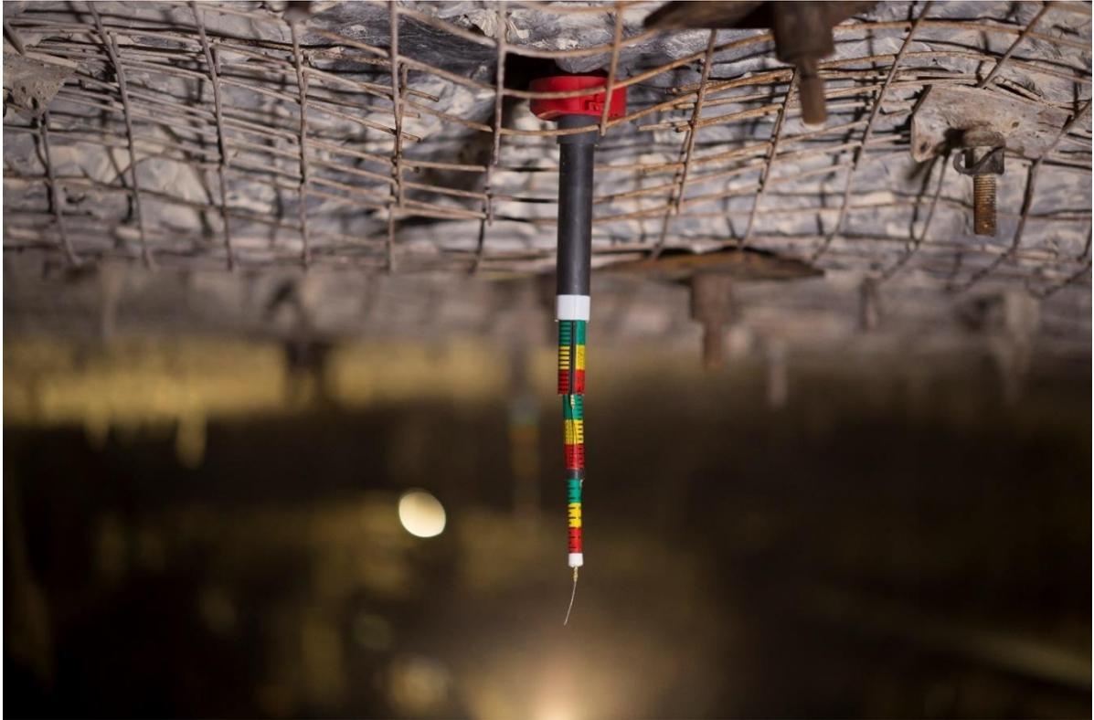
**A view of the extensometer installed in the roof of Bw-1n roadway in Budryk coal mine**
