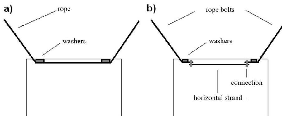
Fig. 3.17. Typical scheme of bolting-strand support: a – monopartial, b – three-partial [101]
