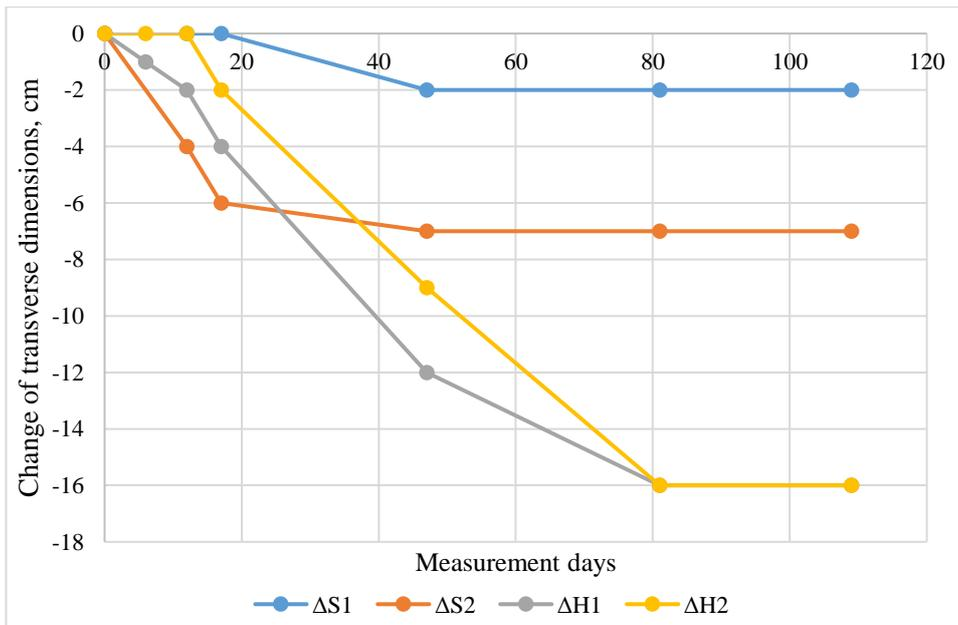
Fig. 12.32. Change of the working transverse dimensions – convergence measuring station No. 4 [135]
