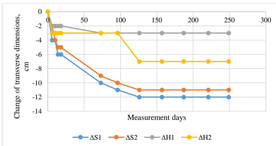
Fig. 12.30. Change of the working transverse dimensions – convergence measuring station No. 2 [135]
