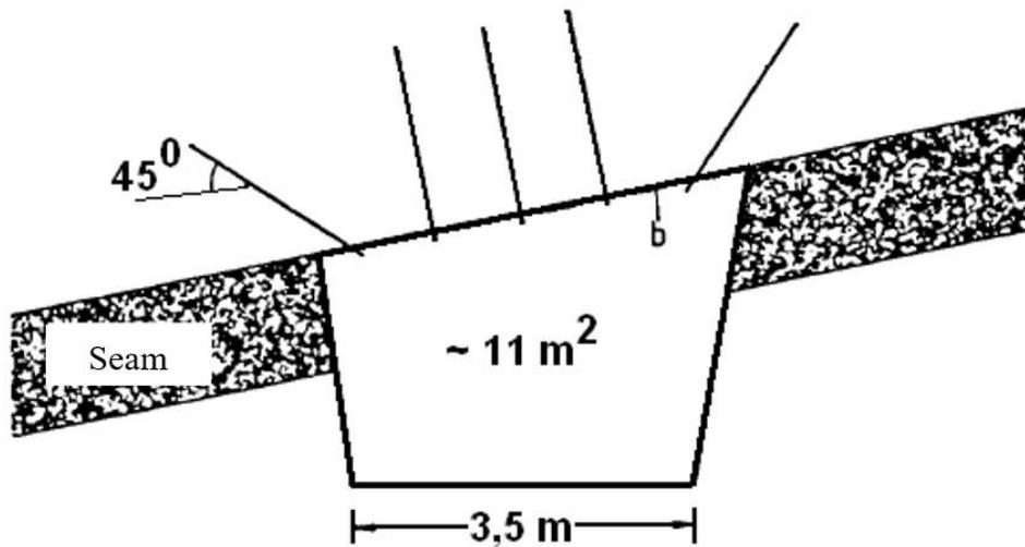
Fig. 3.5. Roadway in the independent bolting support – the fifties [57]
