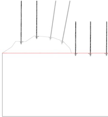
Fig. 11.8. Installation method of lining mesh in the case of caverns occurrence in the roof
