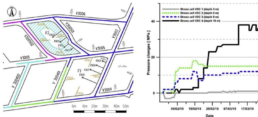
Fig. 3.4. Measurement results of stresses in the V2 pillar [51]
