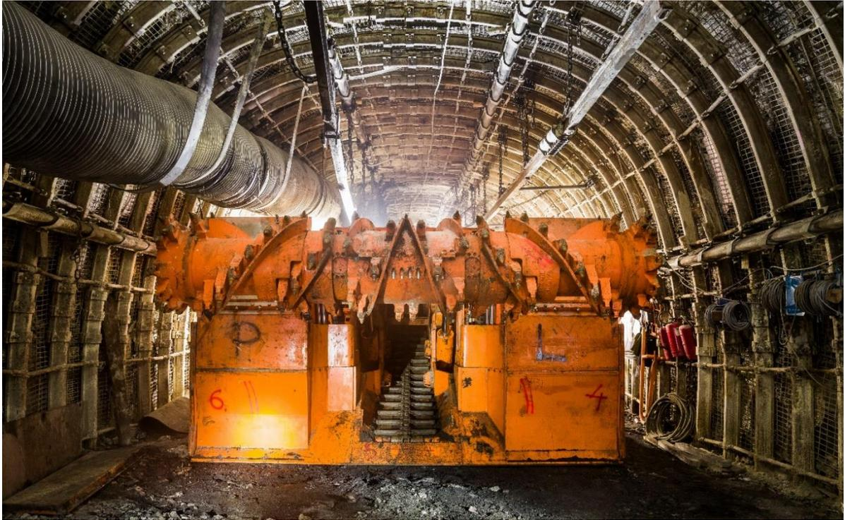
**A view of the Bolter Miner 12CM30 assembled in the Budryk coal mine**
