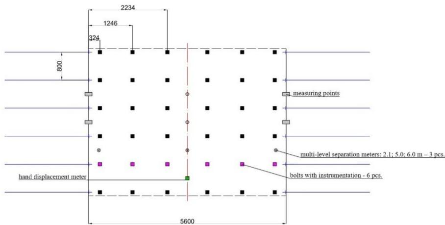
Fig. 12.2. Scheme of a periodical control station – station No. 1 – top view
