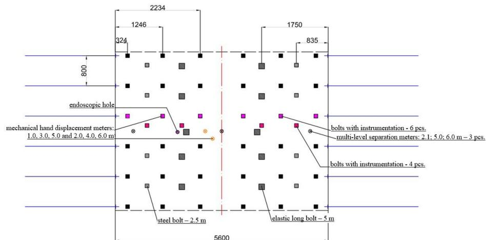
Fig. 12.11. Scheme of the periodical control station – station No. 5 - top view
