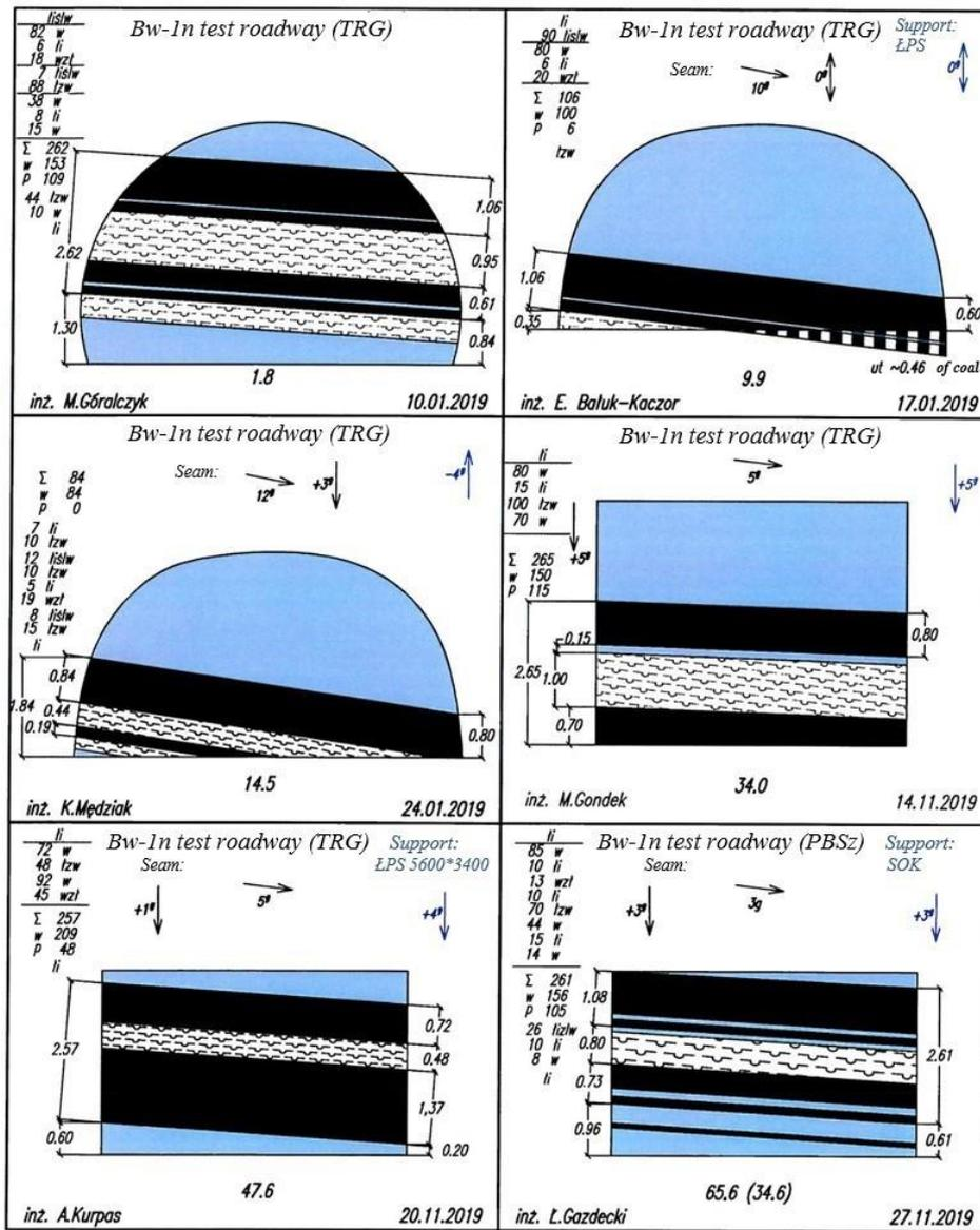
Fig. 8.3. Geological cross-sections of the face 10.01.2019 – 27.11.2019 [135]
