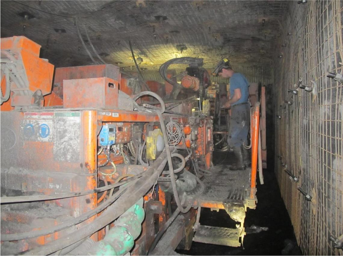
**A view of the conveyor end of the Bolter Miner 12CM30 in Bw-1n roadway in Budryk coal mine**
