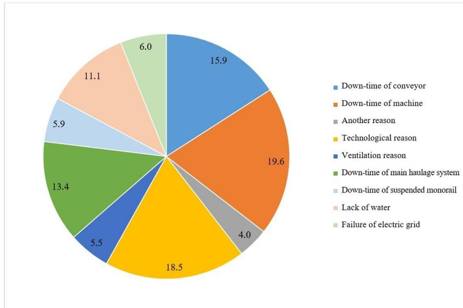
Fig. 14.27. Percentage share in the time of down-times according to the reason
