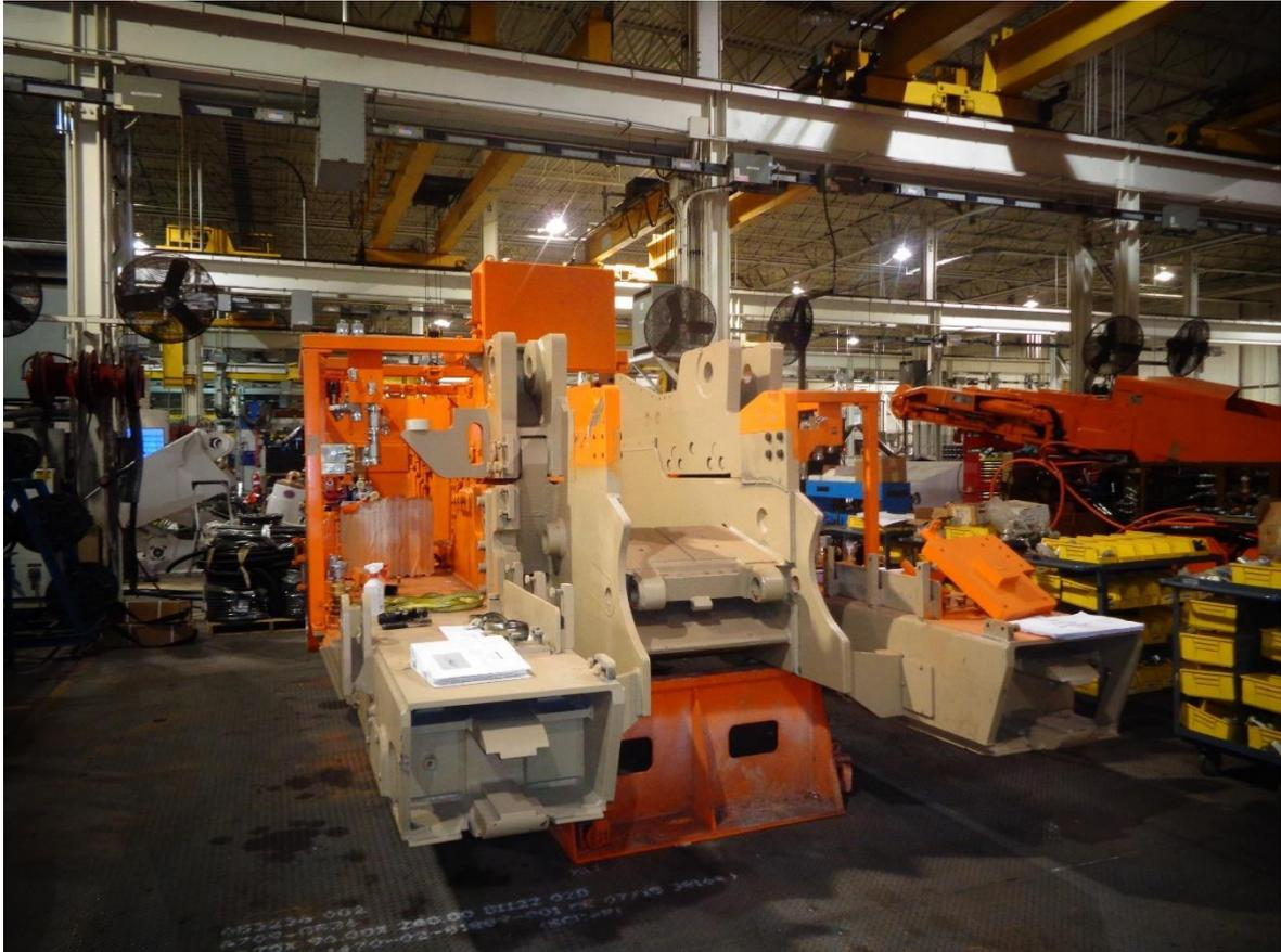
**A view of the main frame of the Bolter Miner 12CM30 in a factory in USA**
