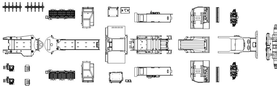
Fig. 11.2. Preparation method of subassemblies of the JOY 12CM30 machine for an assembly [130]
