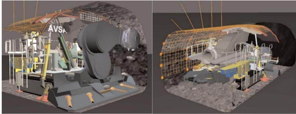
Fig. 2.5. Machine of AVSA type for driving galleries [12]
