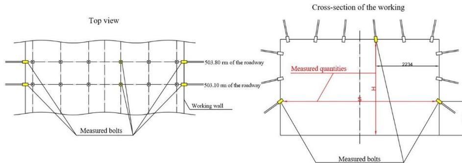
Fig. 12.15. Scheme of the working convergence measurement – station No. 4
