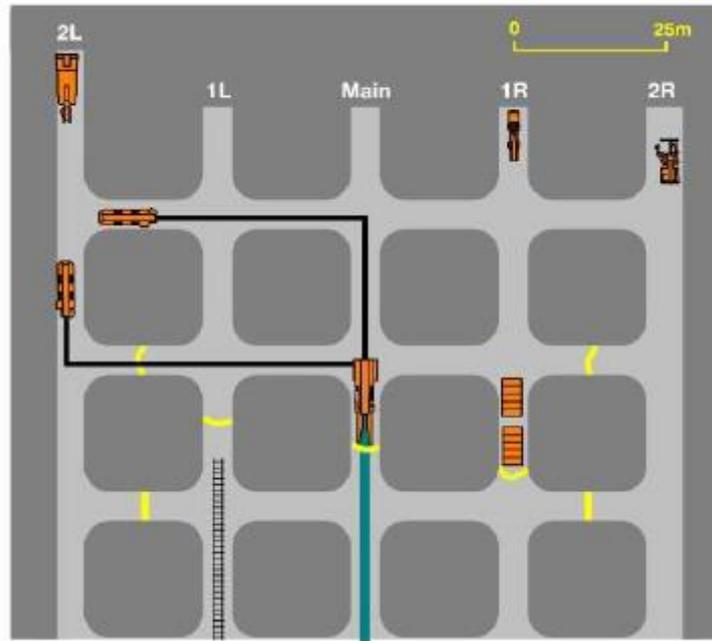
Fig. 3.24. Room-and-pillar system in the Indian hard coal mine [116]
