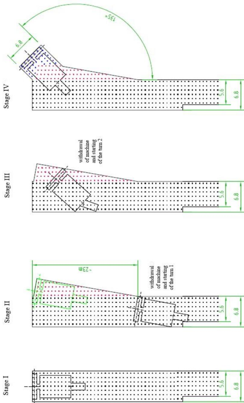
Fig. 13.17. Schematic diagram of driving the bend in the crossing No. 2 according to the Author's conception (turn 135°, departure from the bend of 6.8 m width)
