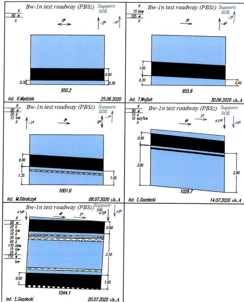
Fig. 8.9. Geological cross-sections of the face 25.06.2020-20.07.2020 [135]
