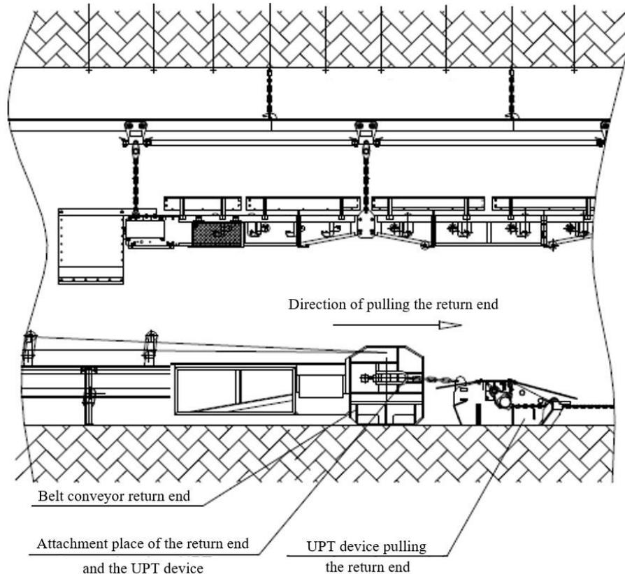
Fig. 11.7. Pulling method of the conveyor return end with use of the UPT device [135]
