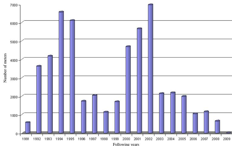
Fig. 3.2. Length of workings driven in independent roof bolting system in the years 1991÷2009 [45-46]
