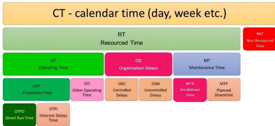
Fig. 2.3. Structure of the calendar time of roadway working acc. to Australian views [9]
