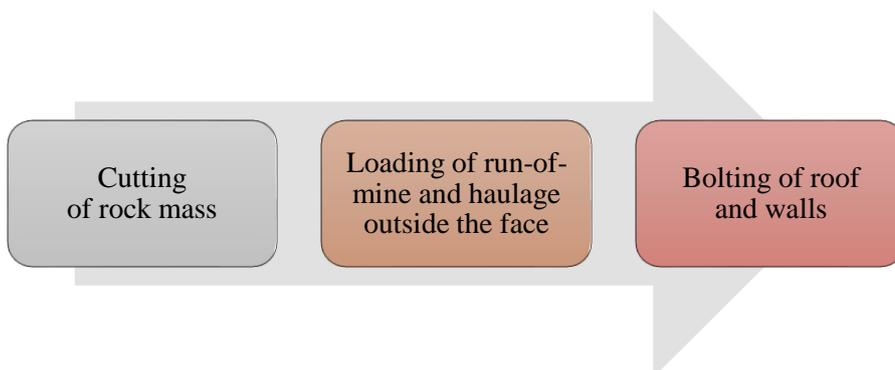
Fig. 2.6. Basic operations connected with a roadway drivage with use of Bolter Miner
