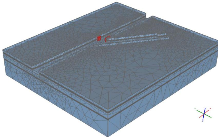
Fig. 10.3. Three-dimensional model of the rock mass acc. to GiG – support of the bend No. 2 [136]
