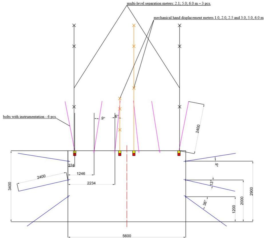
Fig. 12.6. Scheme of a periodical control station – station No. 3 – vertical section
