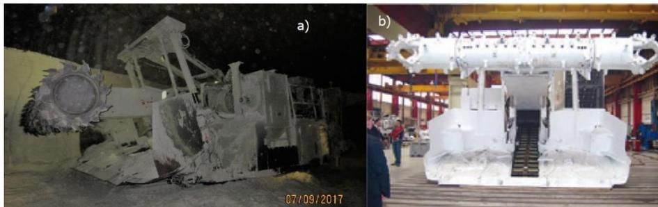
Fig. 2.16. MB670 Bolter Miner in salt mines: a) applied for an exploitation of rock-salt in the Polkowice-Sieroszowice cooper-ore mine belonging to the Polish KGHM, b) prepared for an operation in one of the German mines of potassic salts
