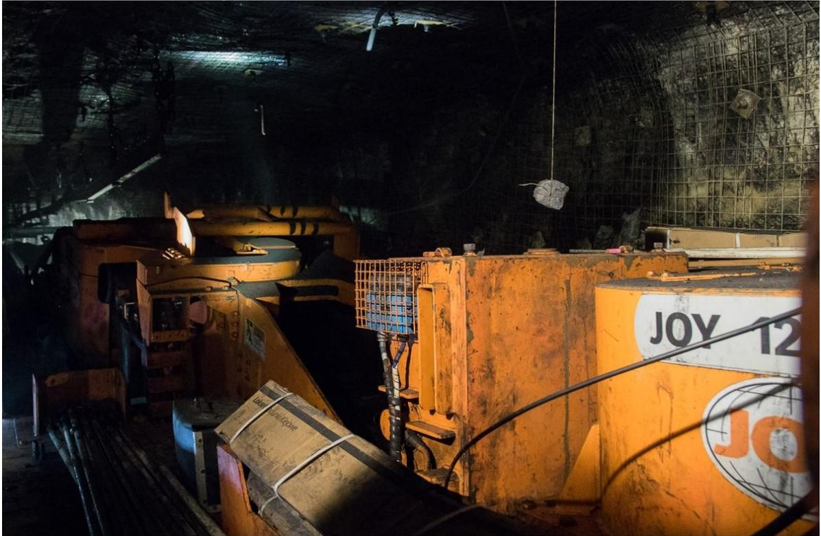
**A view of the Bolter Miner 12CM30 in the face of Bw-1n roadway in Budryk coal mine**
