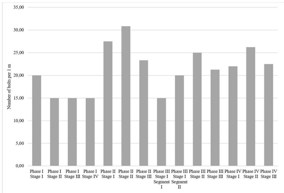
Fig. 11.21. Total number of bolts falling to 1 m of the working at individual driving stages of the Bw-1n test roadway
