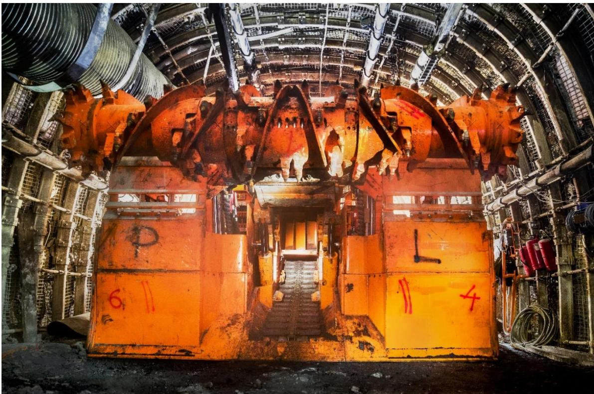
**A view of the Bolter Miner 12CM30 assembled in the undergrounds of the Budryk mine – for the first time in history of Polish coal mining industry**
