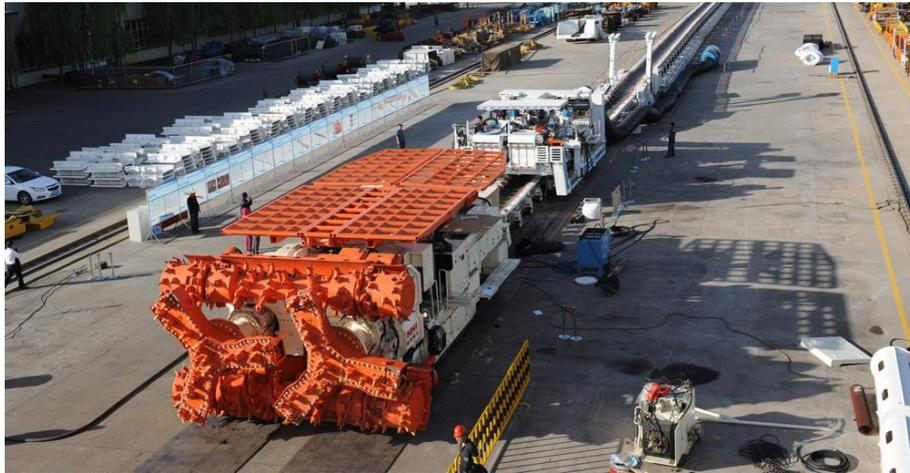
Fig. 2.14. Full-face QMJ4260 machine for rapid driving of coal roadways with mobile multi-head bolter in the Daliuta mine [32]
