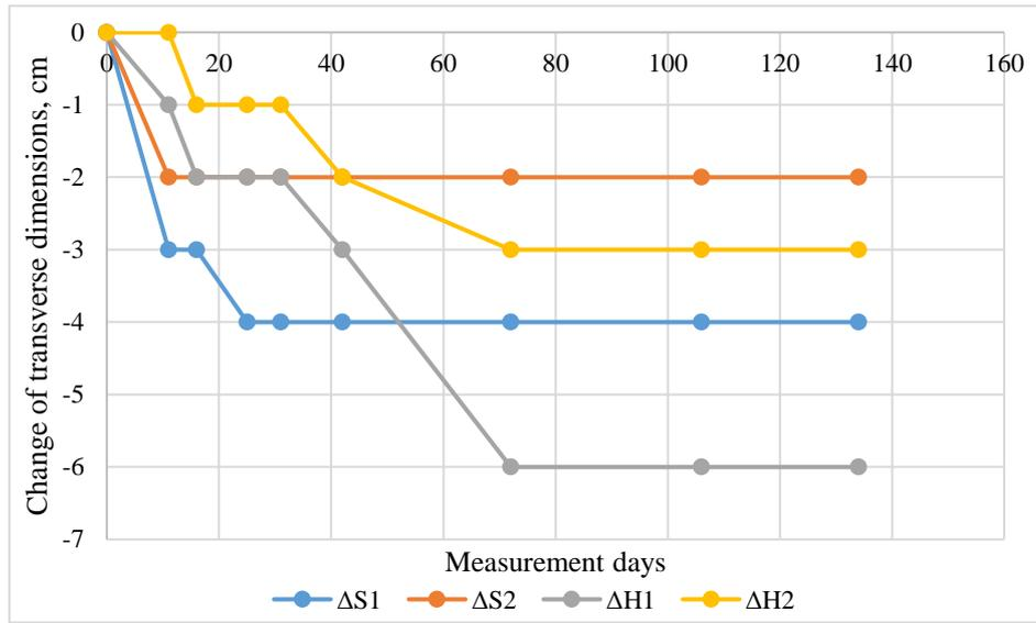
Fig. 12.31. Change of the working transverse dimensions – convergence measuring station No. 3 [135]
