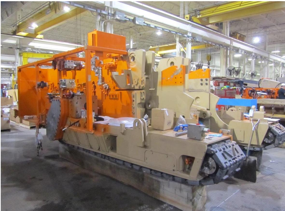
**Bolter Miner 12CM30 during its assembly in US factory**
