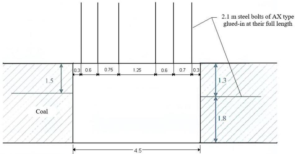
Fig. 3.15. An example of the scheme of independent bolting support – Angus Place mine, Western Coal Field, New South Wales, Australia [96]
