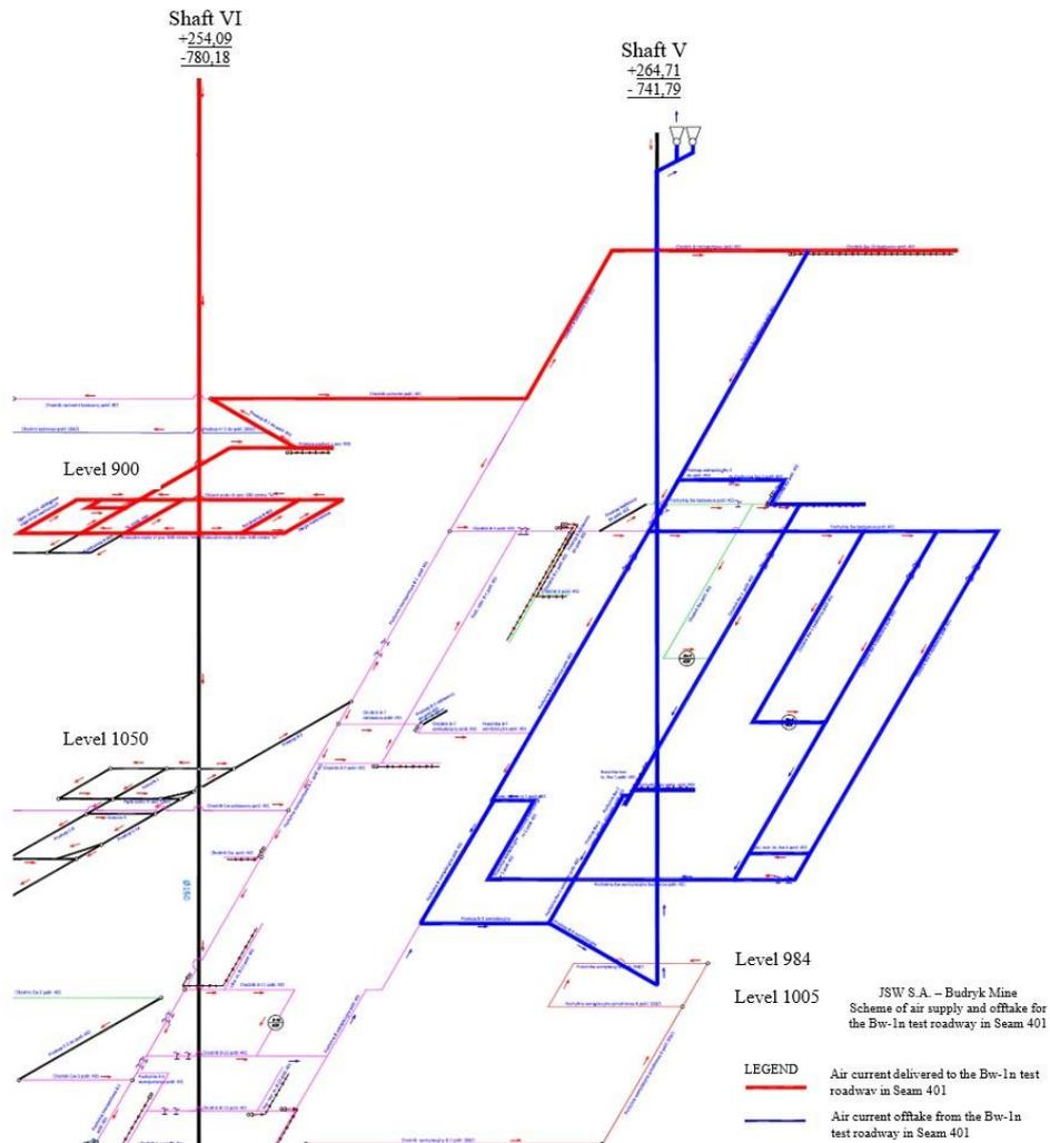
Fig. 11.24. System of air supply and offtake from the Bw-1n test roadway [135]
