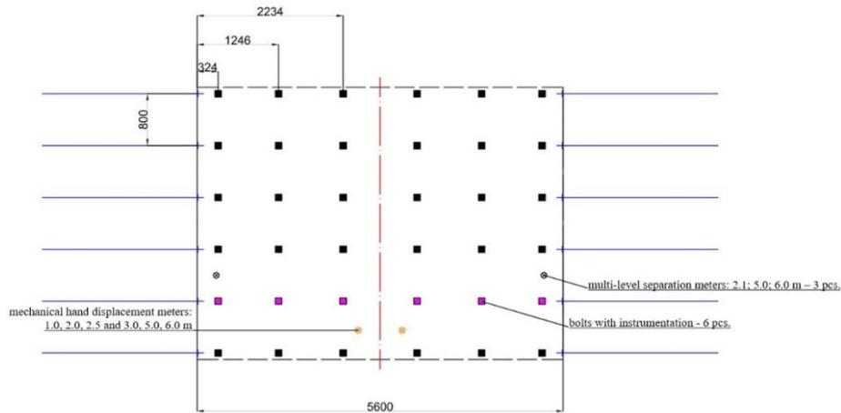
Fig. 12.7. Scheme of a periodical control station – station No. 3 - top view
