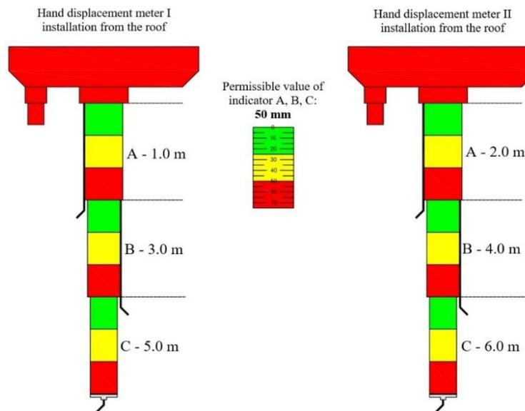
Fig. 12.5. Scheme of the mechanical hand displacement meter
