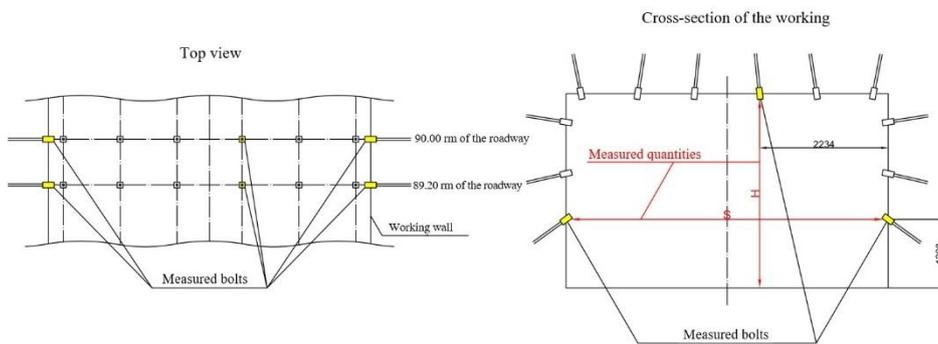
Fig. 12.13. Scheme of the working convergence measurement – station No. 2
