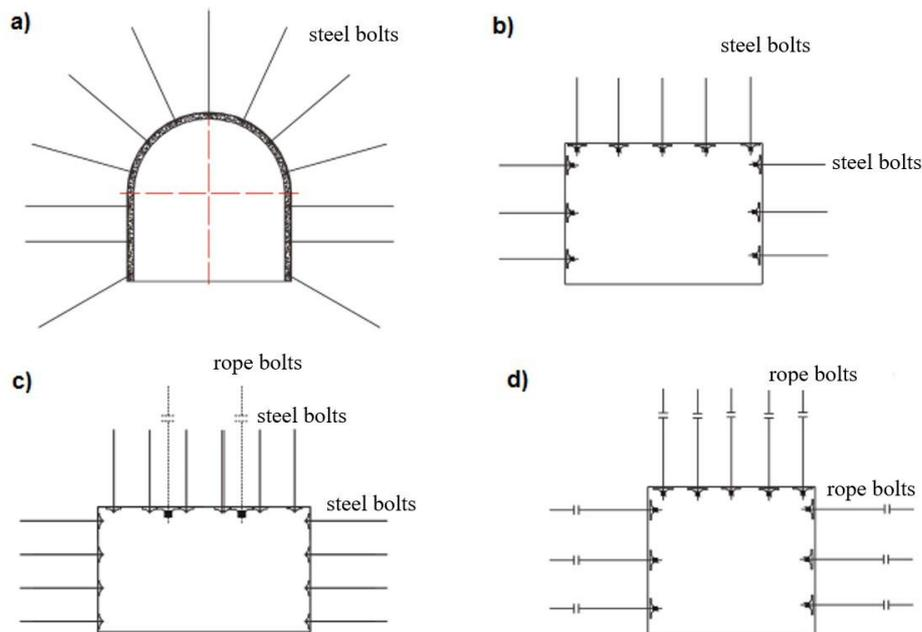
Fig. 3.20. Basic schemes used in Chinese hard coal mines: a) steel bolts and shotcrete, b) steel bolts, c) steel and rope bolts, d) rope bolts [83]
