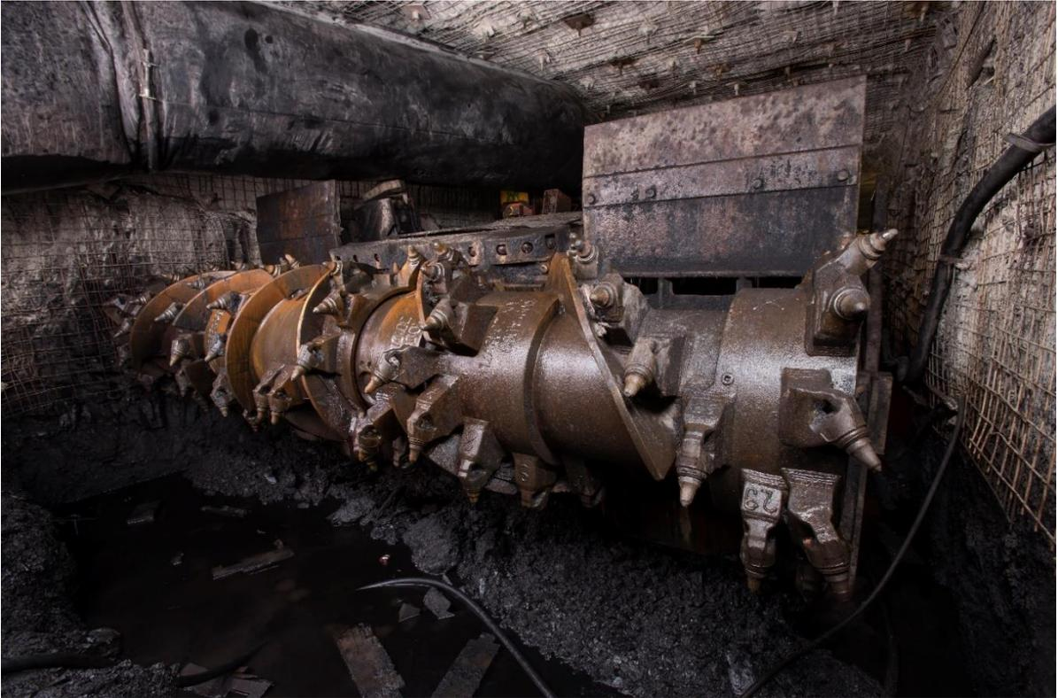
**A view of the cutting head of the Bolter Miner 12CM30 in the face of Bw-1n roadway in Budryk coal mine**
