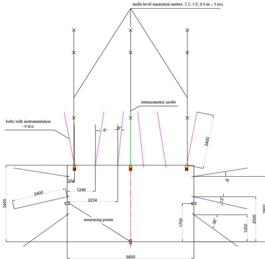
Fig. 12.1. Scheme of a periodical control station – station No. 1 – vertical section
