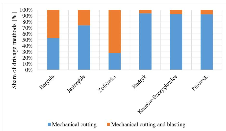
Fig. 6.2. Percentage share of roadway workings length in individual mines of the JSW S.A. over the years 2017-2018
