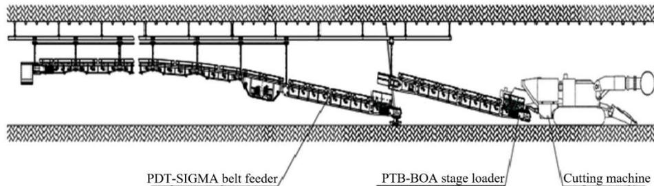
Fig. 2.10. The run-of-mine haulage system from the face driven with the 12CM30 Komatsu Bolter Miner machine in one of the Polish mines with use of suspended belt conveyors
