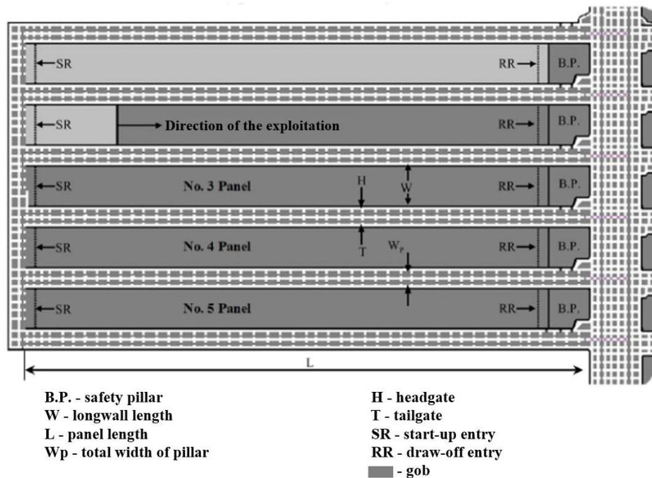
Fig. 3.12. Typical scheme of the exploitative panel development in the United States [6]
