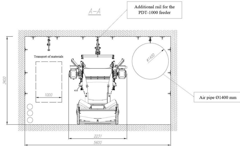
Fig. 11.22. Cross-section of the working with installed air pipe Ø1400 mm [135]
