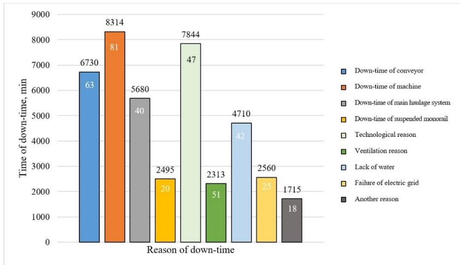
Fig.14.25. Time of down-times over the period of 10 months of the "Independent Roof Bolting Support" project realization with a specification of reasons
