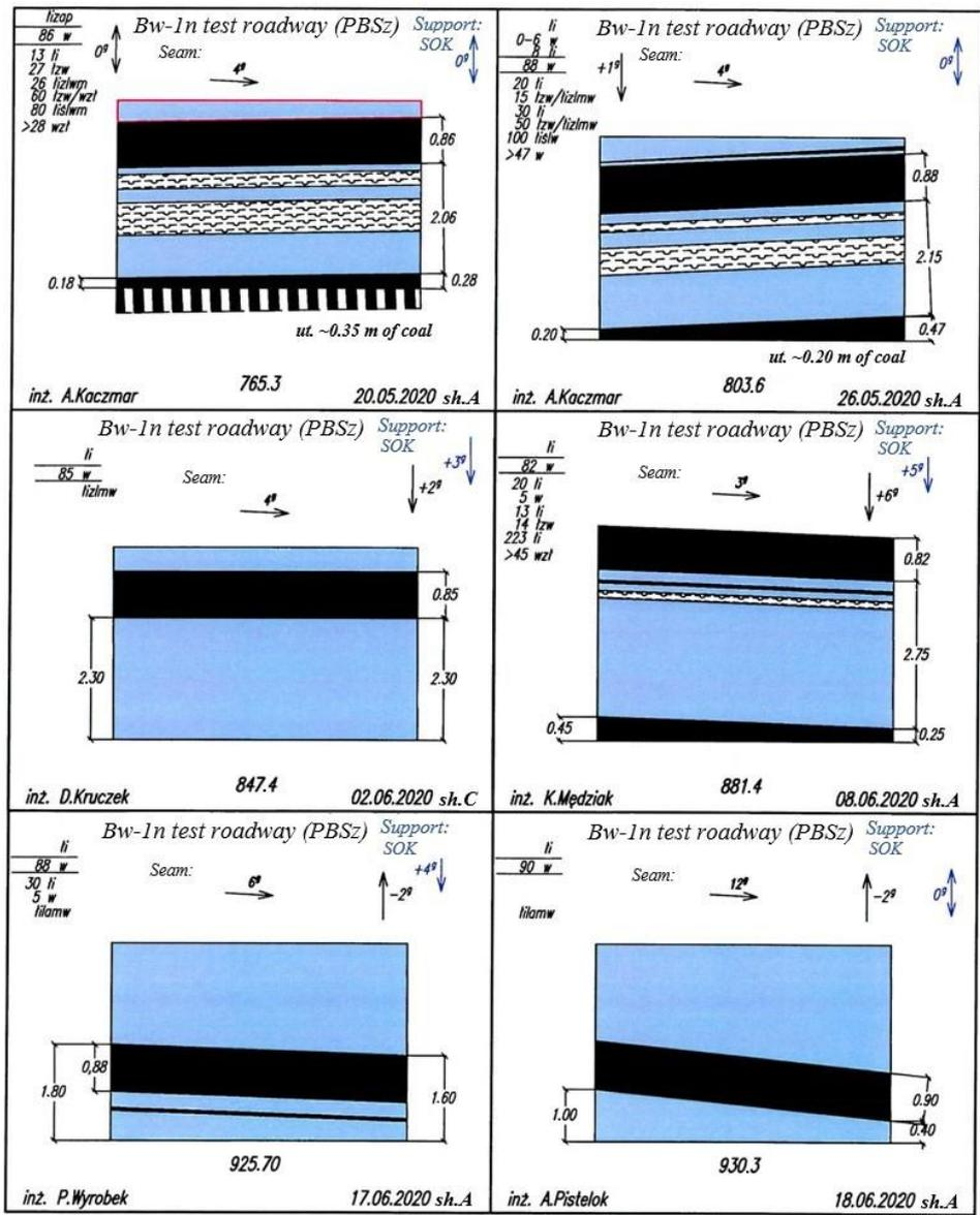
Fig. 8.8. Geological cross-sections of the face 20.05.2020 – 18.06.2020 [135]
