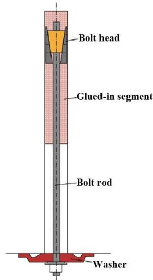
Fig. 3.13. Mechanical bolt with glued-in segment [83]
