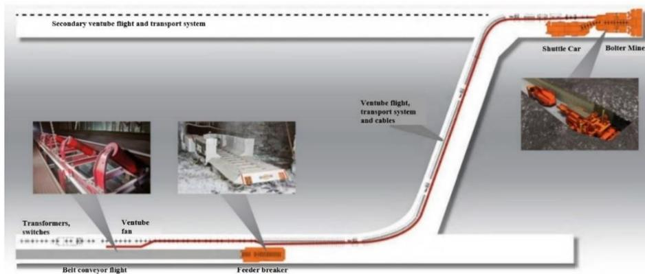
Fig. 2.7. Basic elements of heading face technical system with Bolter Miner machine [8]
