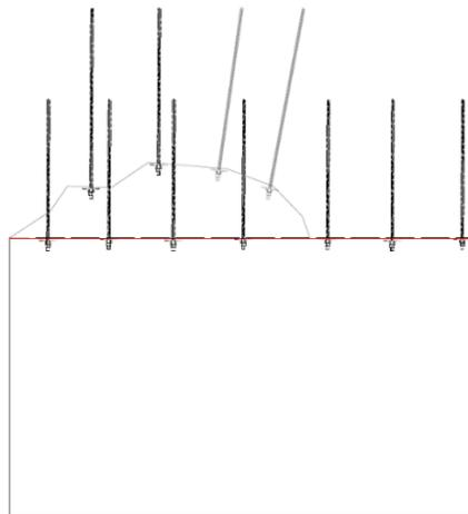
Fig. 11.9. Bolting method of lining mesh in the case of caverns occurrence in the roof
