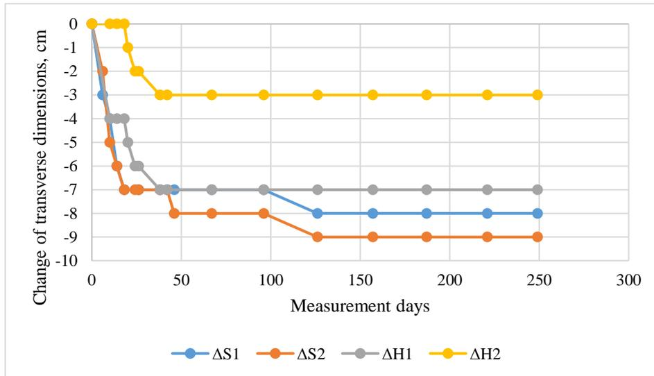
Fig. 12.29. Change of the working transverse dimensions – convergence measuring station No. 1 [135]
