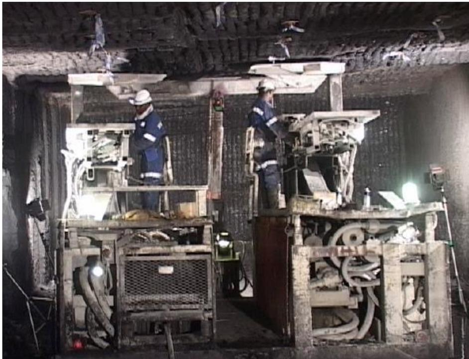
Fig. 3.25. Bolting in the face in a hard coal mine in the Republic of South Africa [119]
