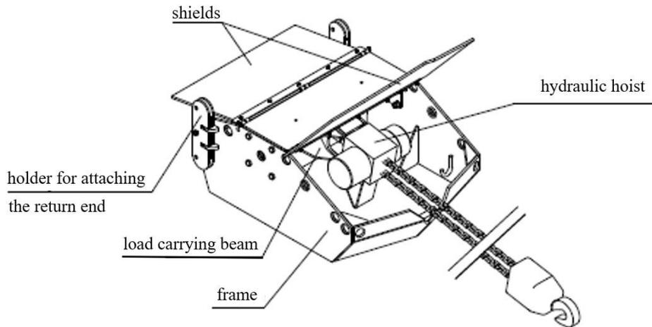
Fig. 11.6. Scheme of the UPT device construction [135]
