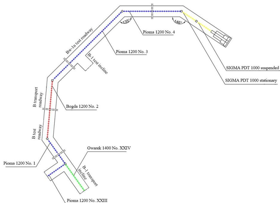
Fig. 11.5. Scheme of haulage equipment configuration after having made the bend No. 2
