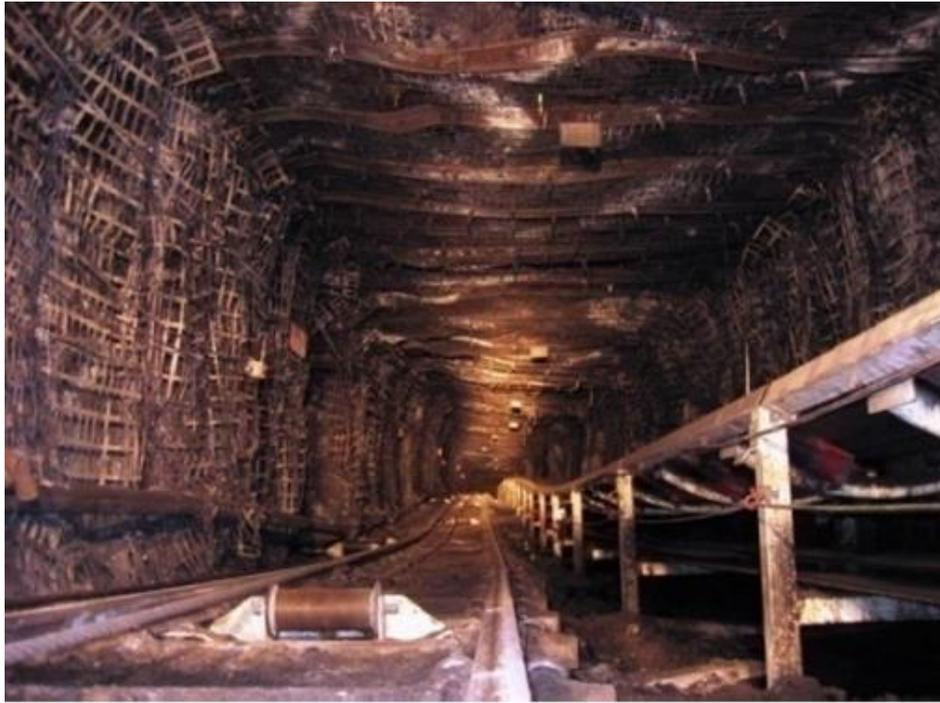
Fig. 3.26. The working driven in independent bolting support in the Iranian Tabas mine [122]
