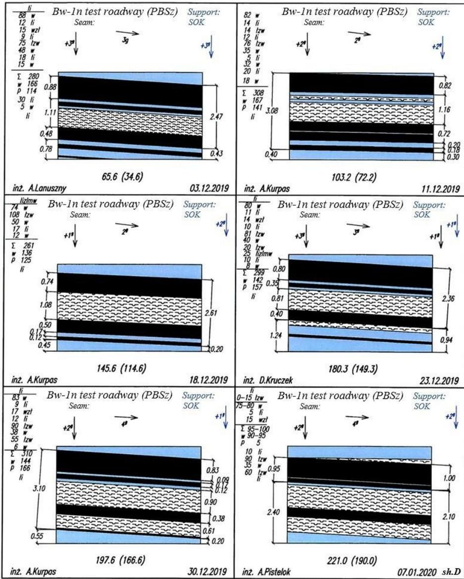
Fig. 8.4. Geological cross-section of the face 3.12.2019 – 7.01.2020 [135]
