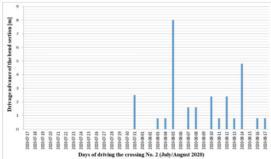
Fig. 13.5. Drivage advance during an execution of the bend (crossing No.2)
