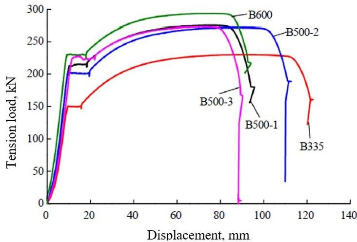
Fig. 3.21. Results of laboratory tests of bolts used in China [107]
