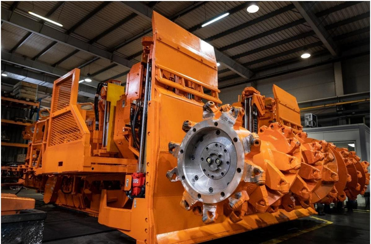
**A cutting head and a loading table of the Bolter Miner 12CM30 assembled in JOY plant in Tychy, Poland**
