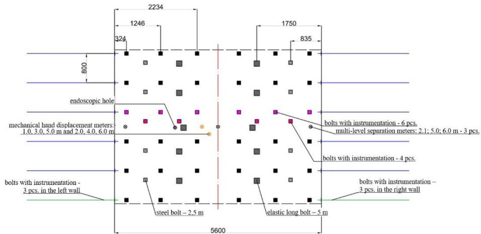
Fig. 12.9. Scheme of periodical control station – station No. 4 – top view
