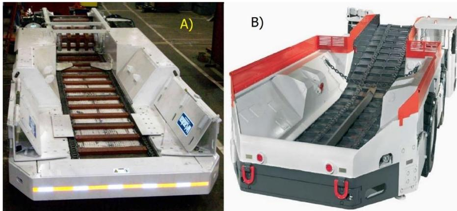
Fig. 2.9. Equipment of the run-of-mine haulage system from the face driven with use of the Bolter Miner: A) discharge – crushing station of Feeder Breaker type, B) vehicle of Shuttle Car type [13]
