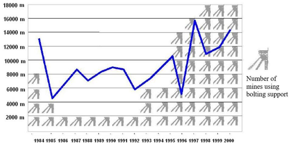
Fig. 3.6. Total metric length of workings in independent bolting support in Germany over the years 1984-2000 [62]
