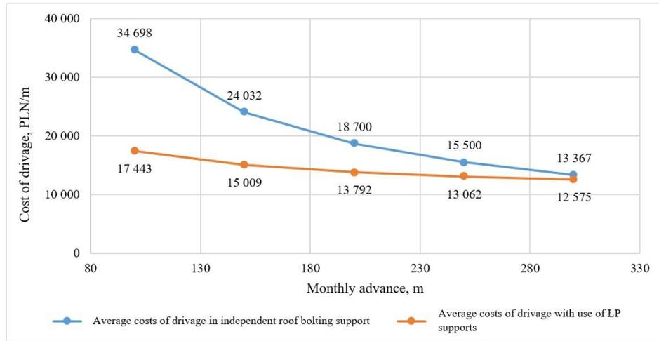
Fig. 14.29. Costs of the working drivage in relation to the monthly advance [128]
