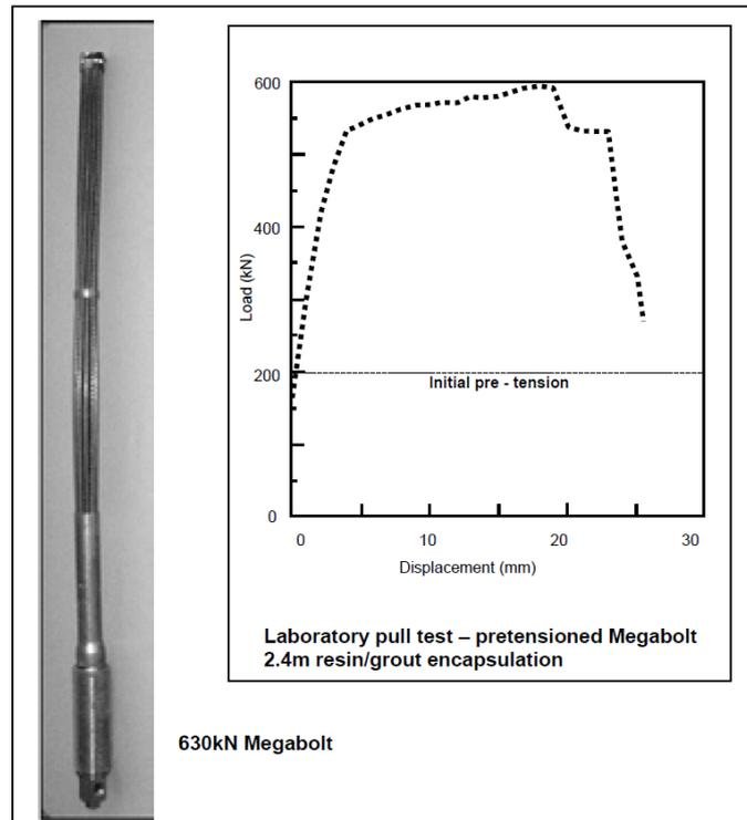
Fig. 3.16. Characteristic of the load-bearing capacity of the 630 kN Megabolt [98]
