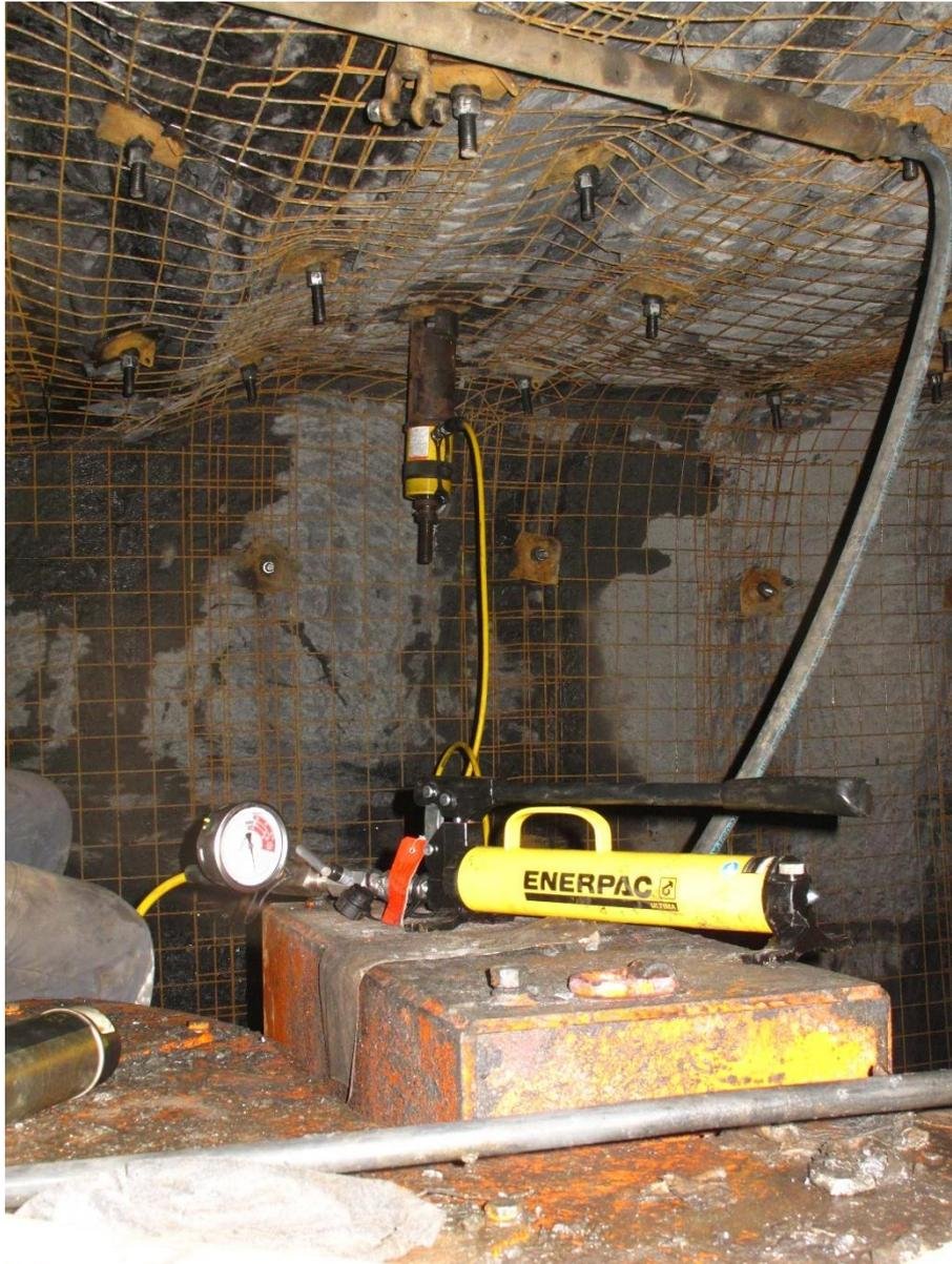
**A view of the pull-out test jack during the test of the bolt in Bw-1n roadway in Budryk coal mine**
