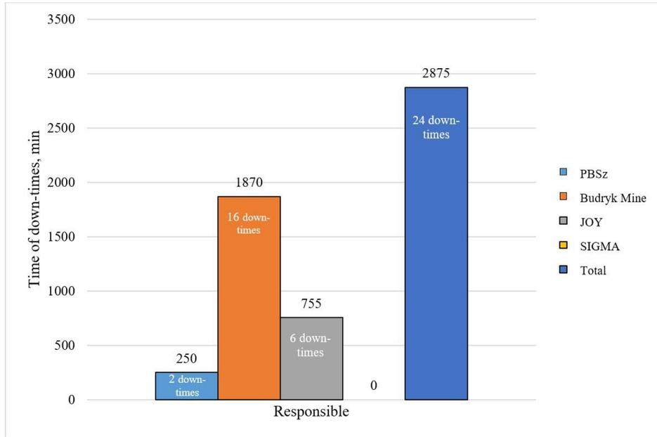
Fig. 14.17. Time of down-times in operation during the sixth month of the project "Independent Roof Bolting Support"
