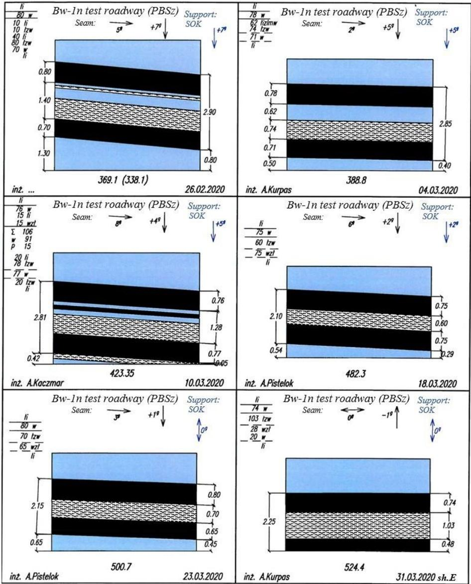
Fig. 8.6. Geological cross-sections of the face 26.02.2020 – 31.03.2020 [135]
