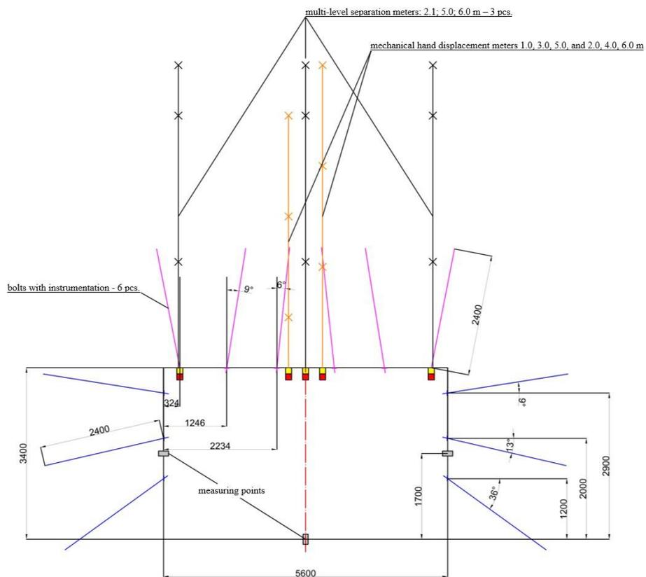
Fig. 12.3. Scheme of periodical control station – station No. 2- vertical section
