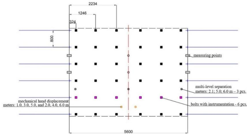
Fig. 12.4. Scheme of periodical control station – station No. 2- top view
