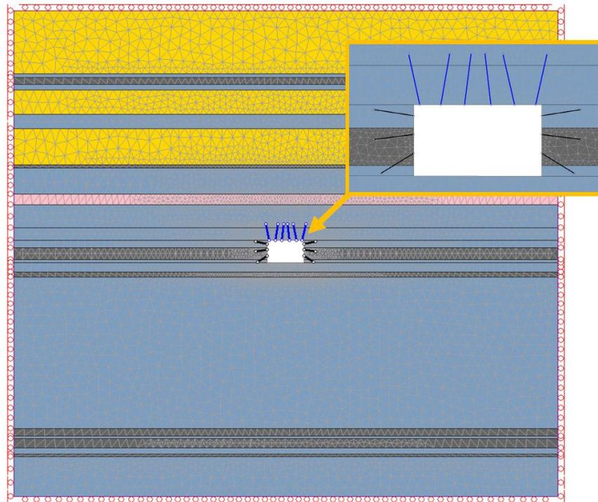
Fig. 10.2. Two-dimensional model of the rock mass acc. to GiG – support of the first straight segment [136]
