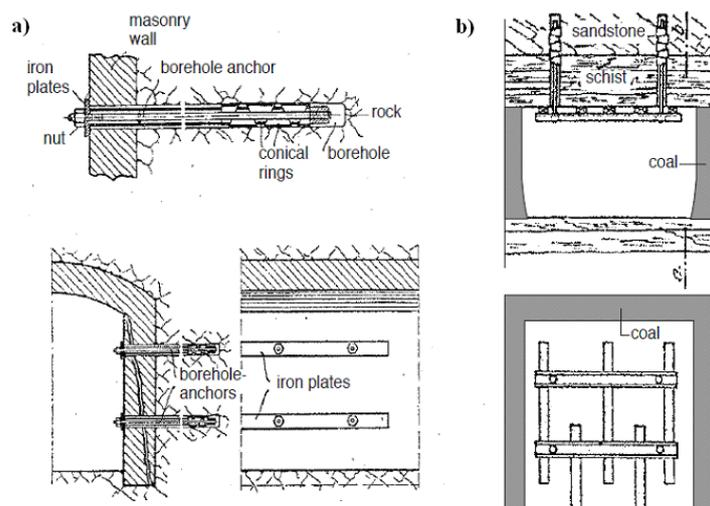
Fig. 3.1. The first application of the bolting support:
