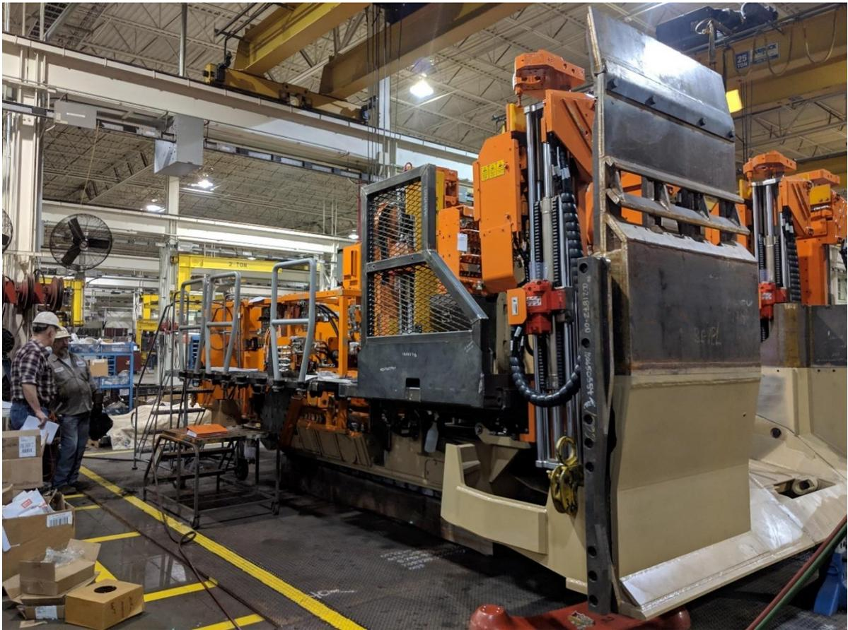
**Bolter Miner 12CM30 during its assembly in a factory in USA**
