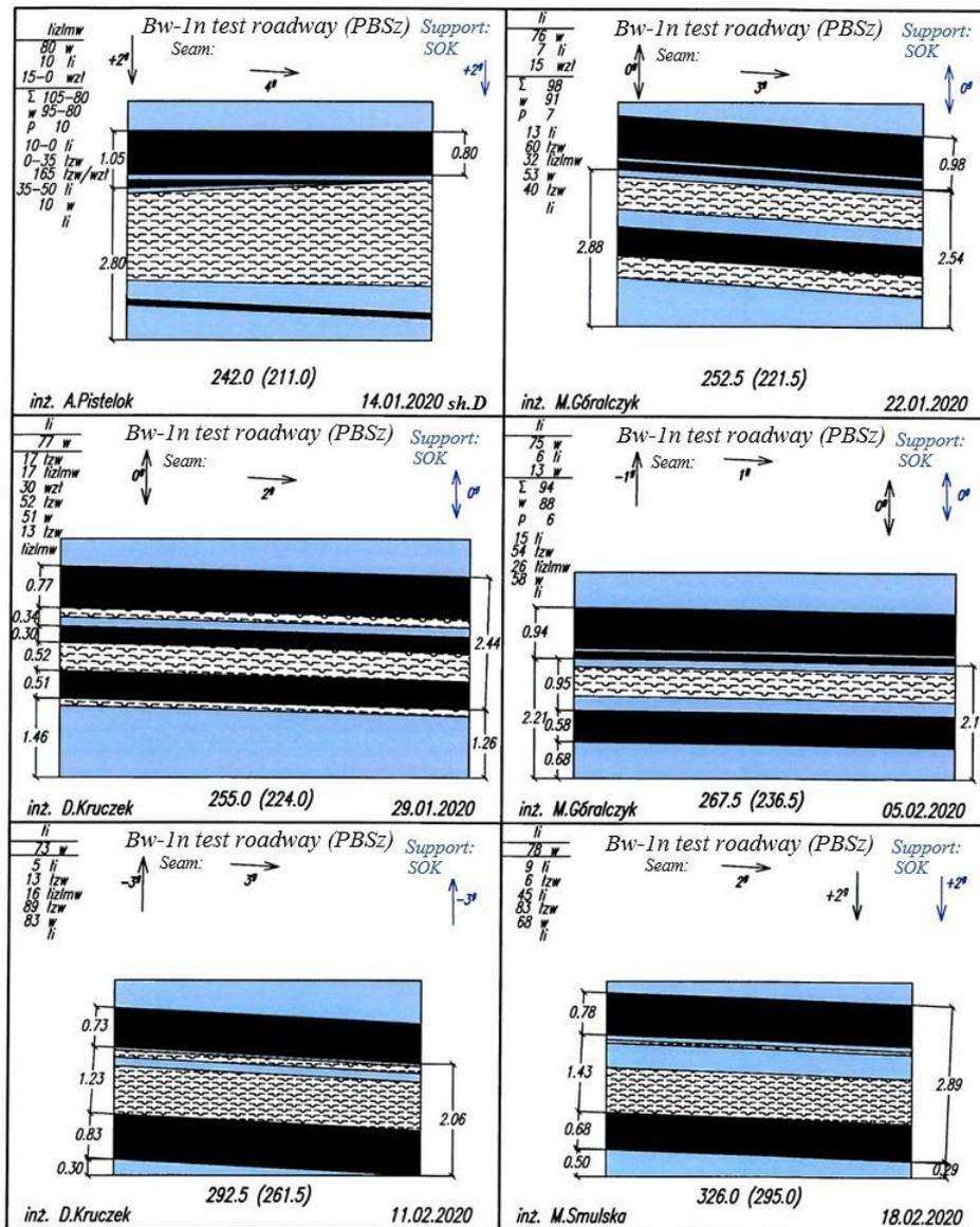
Fig. 8.5. Geological cross-sections of the face 14.01.2020 – 18.02.2020 [135]
