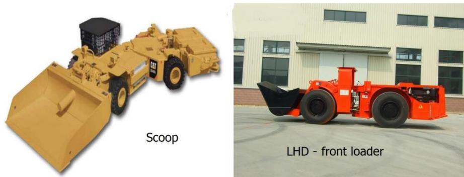
Fig. 2.11. Front loaders (Scoop, LHD) as an auxiliary transport equipment
