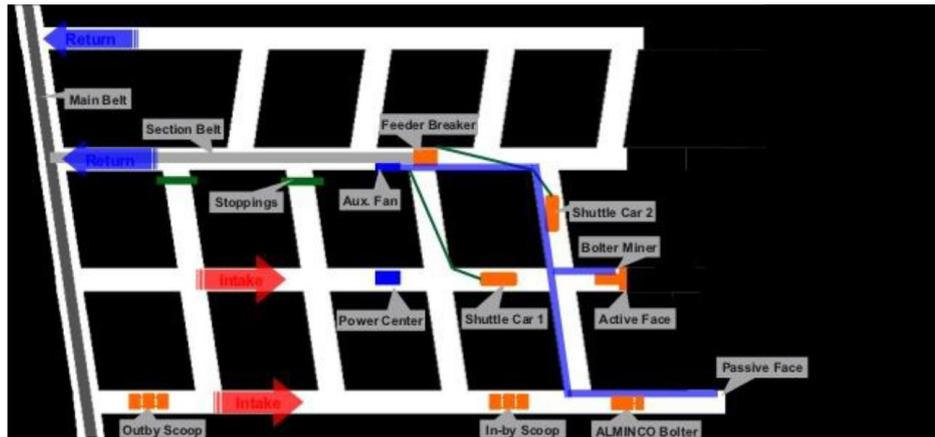
Fig. 2.15. Room-and-pillar mining system with use of the 12CM30 Bolter Miner machine used in the Czech CSM mine [33]
