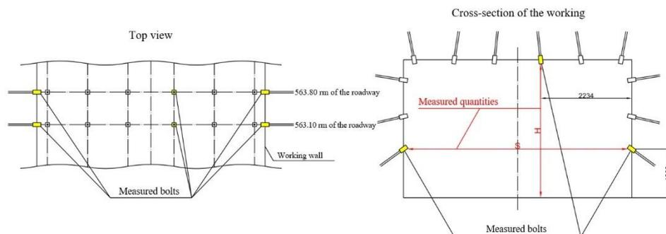
Fig. 12.16. Scheme of the working convergence measurement – station No. 5
