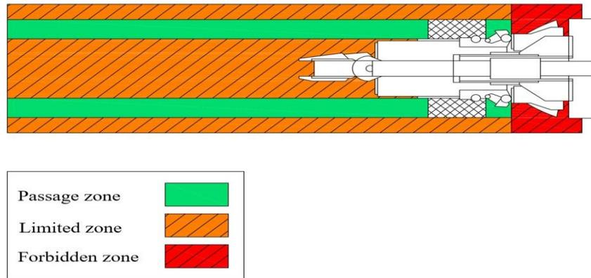
Fig. 11.3. Access zones during an operation of bolters [130]
