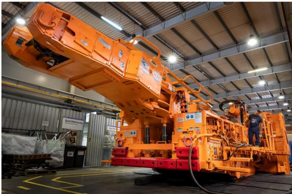
Fig. 6.7. JOY 12CM30 machine in the Komatsu Plant in Tychy – stage loader
