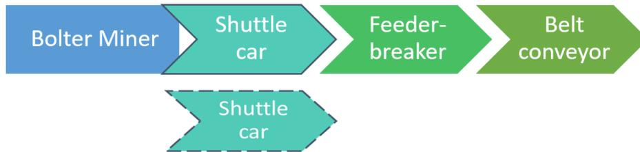
Fig. 2.8. Basic equipment of the face mechanization system with use of Bolter Miner
