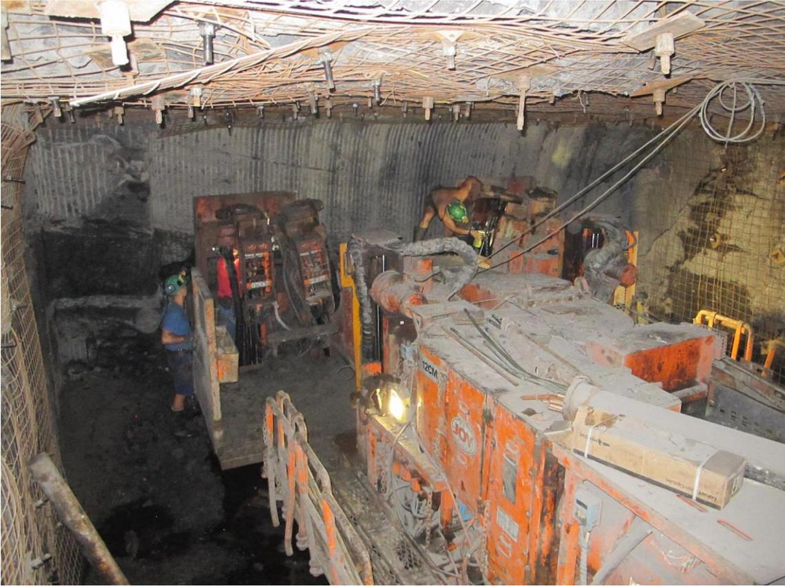
**A view of the Bolter Miner 12CM30 in the face of Bw-1n roadway in Budryk coal mine**
