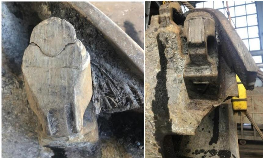
Fig. 13.6. A view of damaged cutter-bar of the 12CM30 cutting drum
