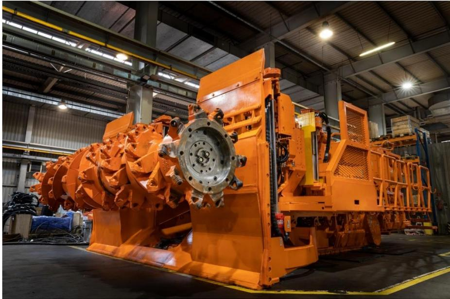
Fig. 6.6. JOY 12CM30 machine in the Komatsu Plant in Tychy – cutting head
