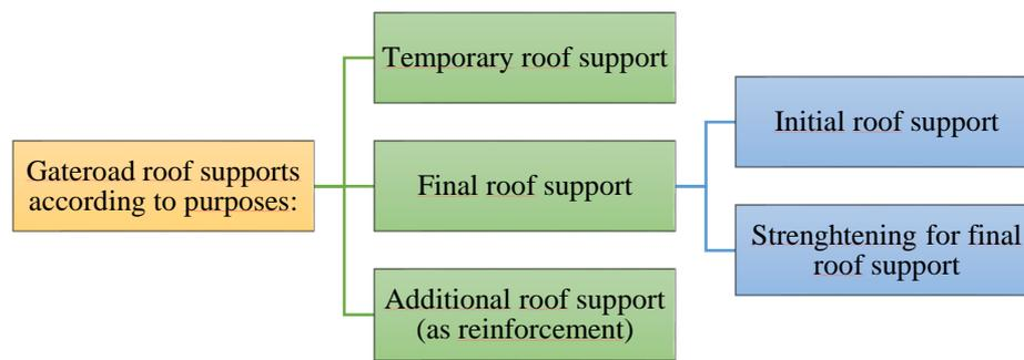
Fig. 2.13. Systematics of gallery supports due to their application and installation time
