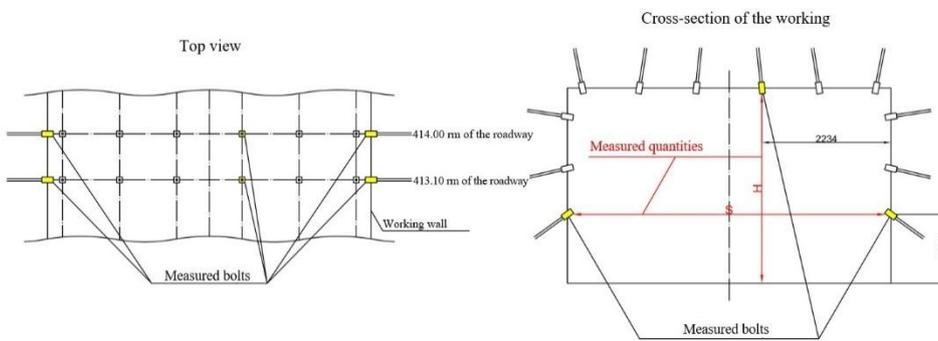
Fig. 12.14. Scheme of the working convergence measurement – station No. 3
