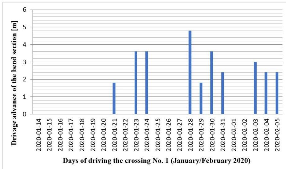
Fig. 13.3. Drivage advance during an execution of the bend (crossing) No. 1
