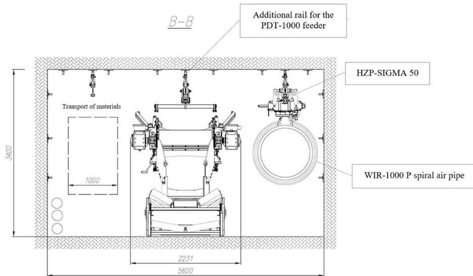
Fig. 11.23. Cross-section of the working with installed WIR-1000P air pipe [135]
