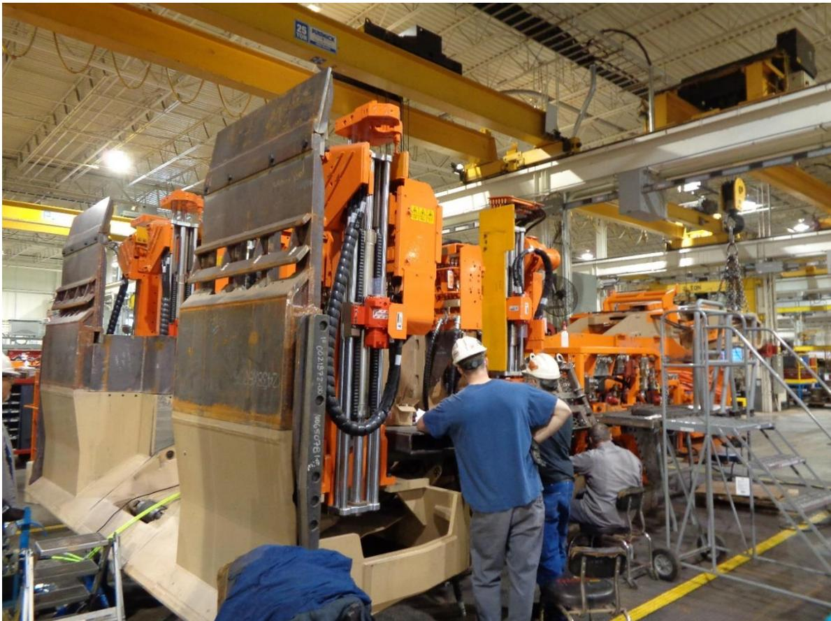
**Assembling of the Komatsu Bolter Miner 12CM30 in a factory in USA**
