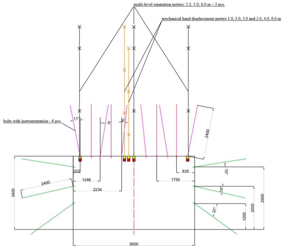
Fig. 12.8. Scheme of a periodical control station – station No. 4 – vertical section
