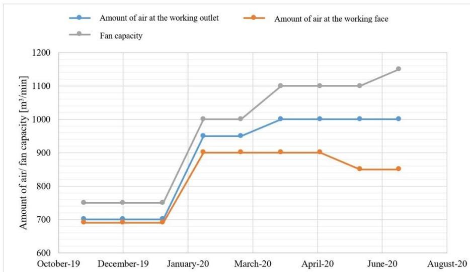
Fig. 11.26. Changeability graph of the air amount and of the fan capacity in the Bw-1n test roadway [135]
