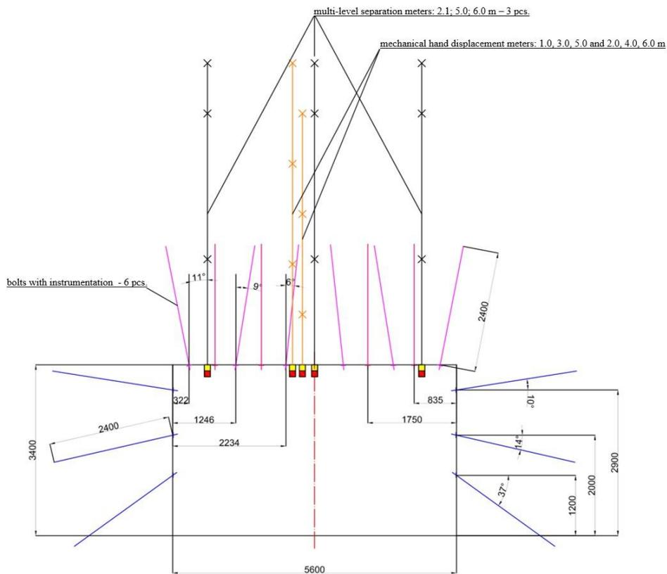
Fig. 12.10. Scheme of the periodical control station – station No. 5 – vertical section
