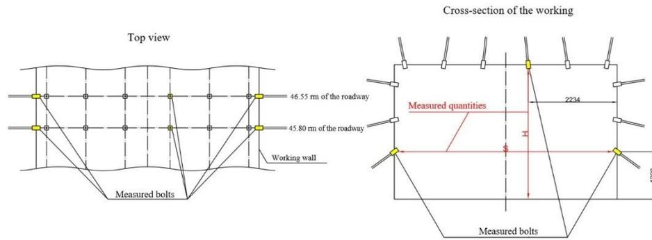
Fig. 12.12. Scheme of the working convergence measurement – station No. 1
