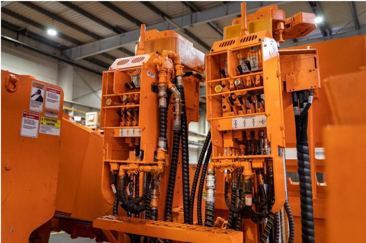
**A view of the hydraulic system steering of the Bolter Miner 12CM30 in JOY plant in Tychy, Poland**
