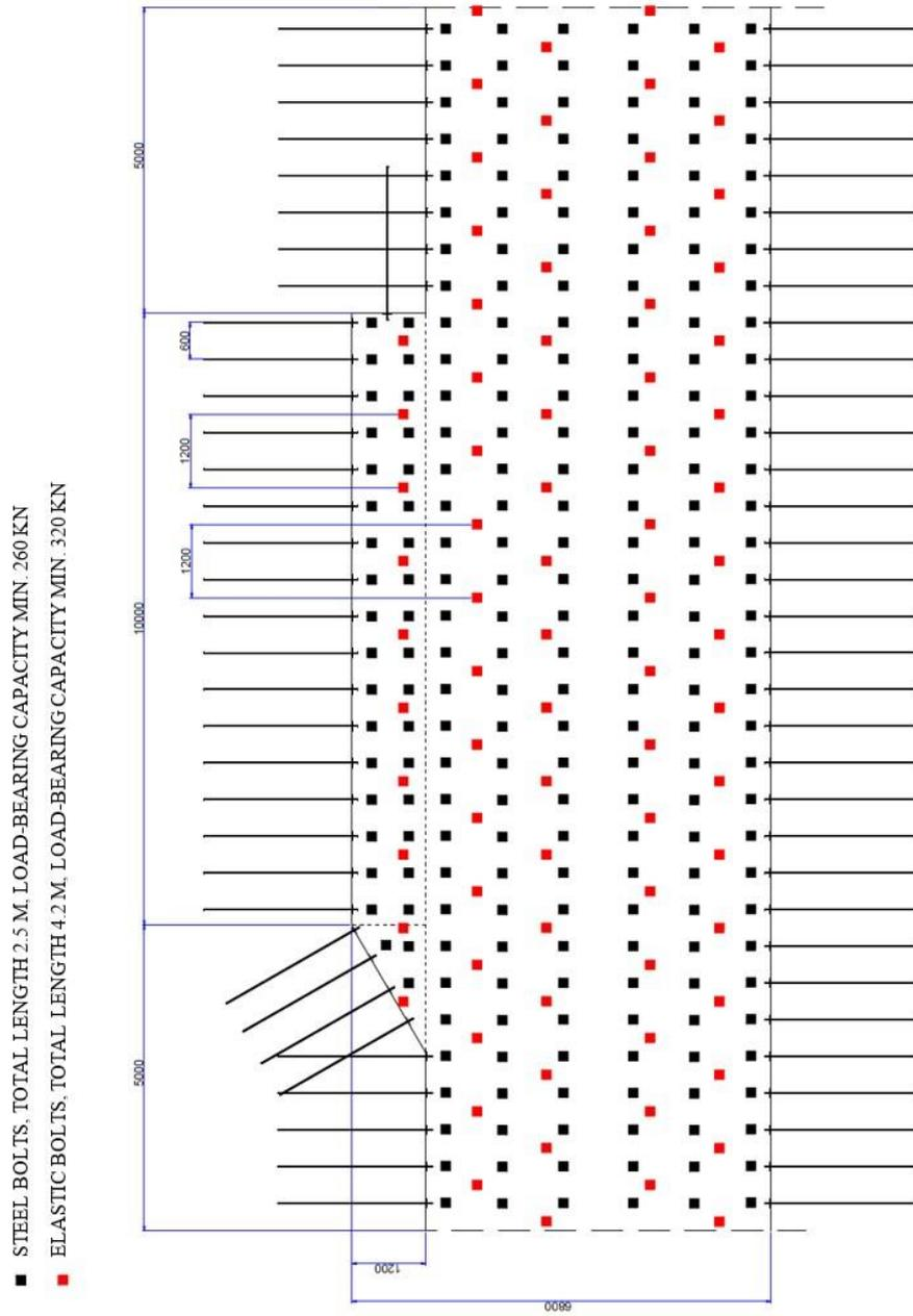
Fig. 11.14. Bolting scheme of an extension for the transformer station before an introduction of changes [135]
