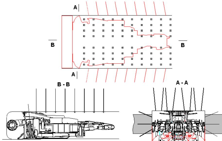
Fig. 3.10. An exemplary bolting scheme in one of the gateroads at the Thoresby mine [72]
